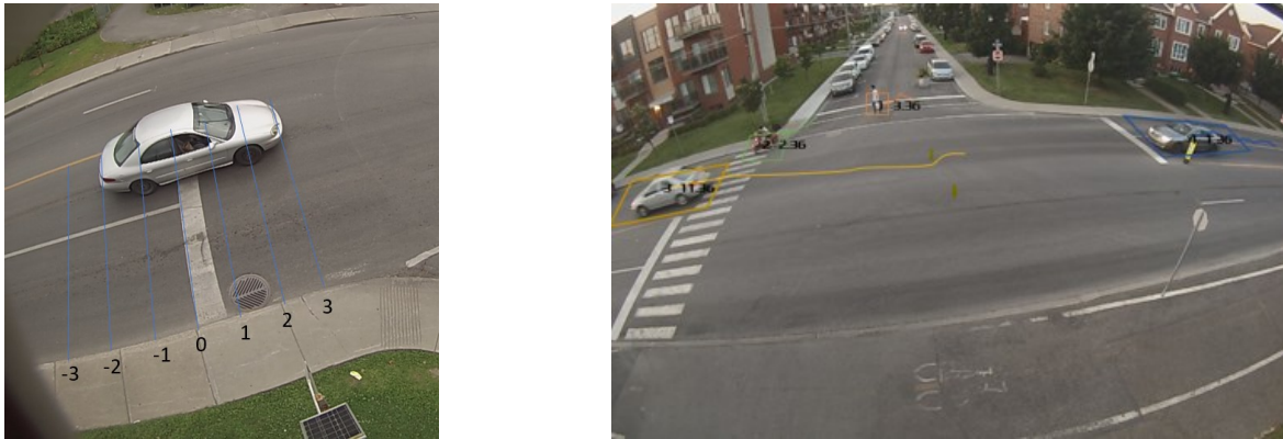
Figure 12 Left, image annotation and labeling at intersection - (westbound Victoria and 28 th avenue), right, examples of video recording presenting road users' tracks, identification number, and speed overlaid (Victoria and 21 st avenue)
