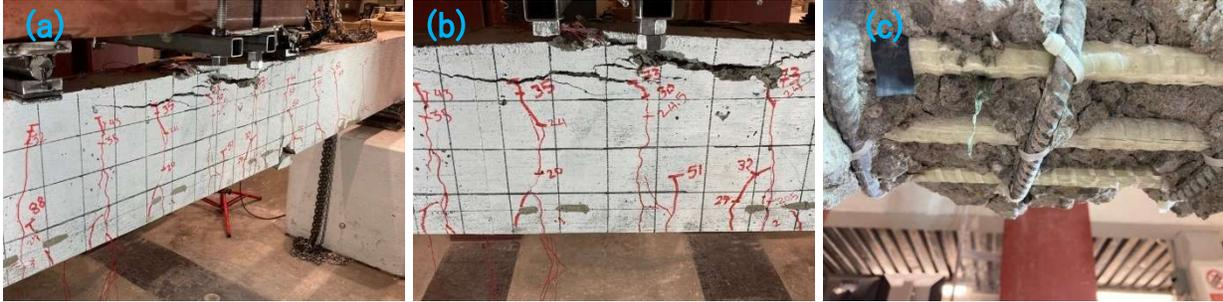
**Figure A.23** Failure of beam confined with transverse reinforcement spacing of 100 mm (a) concrete crushing followed by GFRP rupture; (b) concrete crushing failure; and (c) GFRP bar rupture
