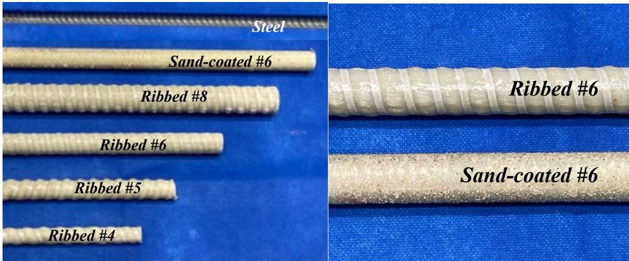
**Figure 4.1** The surface profile of steel, ribbed, and sand-coated Grade III GFRP bars
