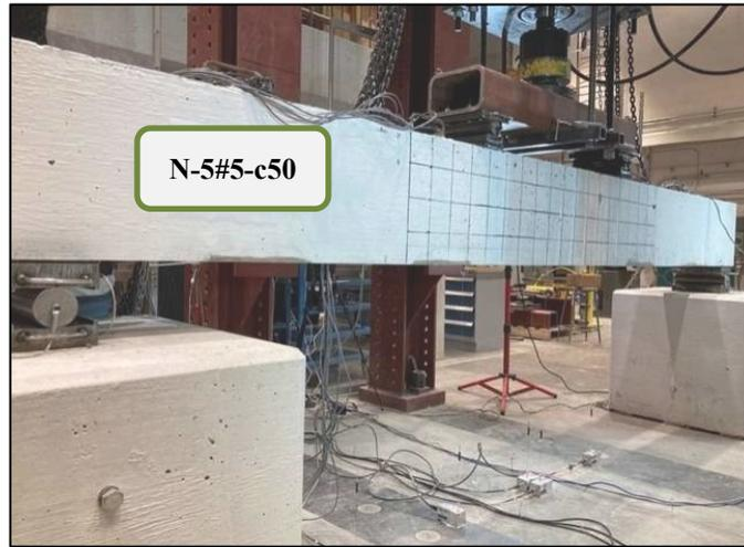
**Figure 6.3** Typical test setup for the tested beams
