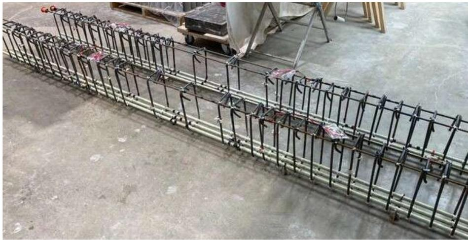
**Figure A.1** Typical GFRP cages for two concrete beams
