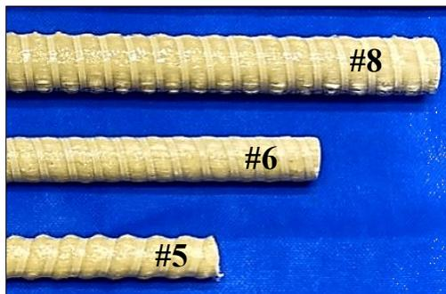
**Figure 6.2** GFRP reinforcement surface configuration
