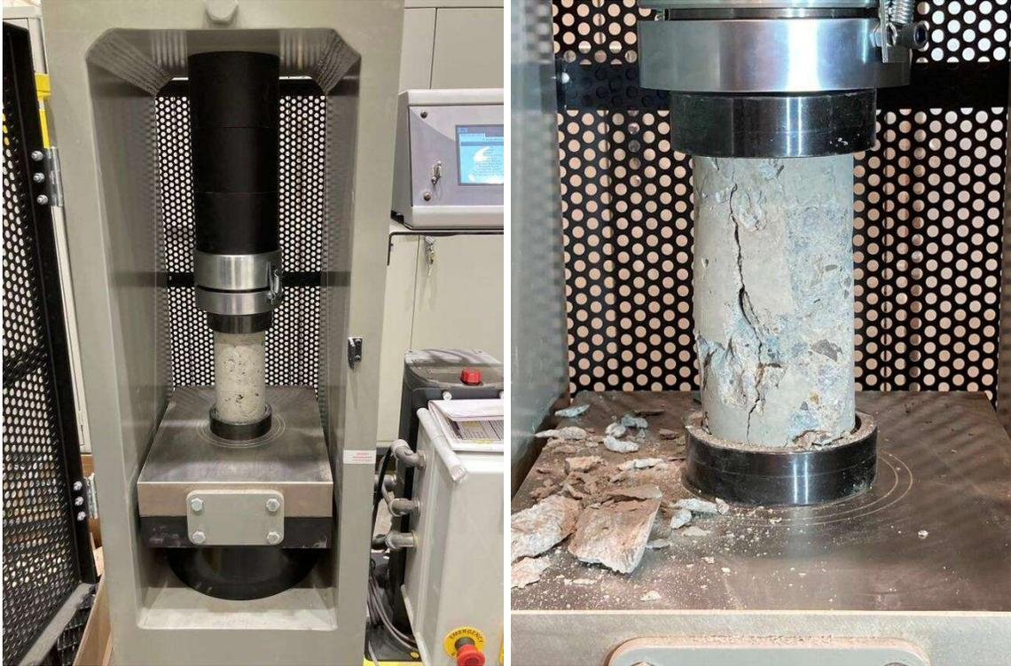
**Figure A.15** Testing concrete cylinders in compression
