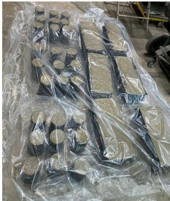
**Figure A.12** Curing of the concrete cylinders and prisms
