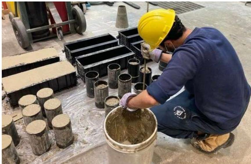
**Figure A.10** Pouring, compacting, and levelling of the cylinders and prisms
