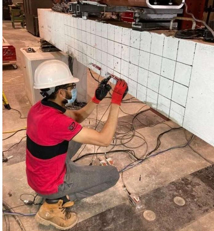
**Figure A.19** Attaching the LVDT to the concrete beam at the crack location
