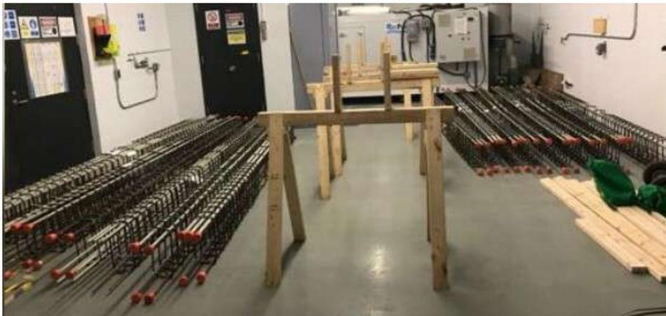
**Figure A.2** GFRP cages for 16 concrete beams
