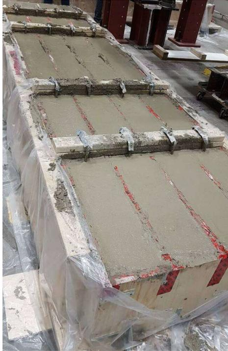
**Figure A.9** Concrete top surface after finished and levelling
