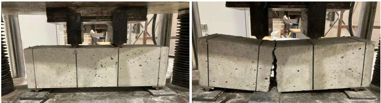
**Figure A.16** Testing the concrete prisms in tension using the four-point bending rupture test
