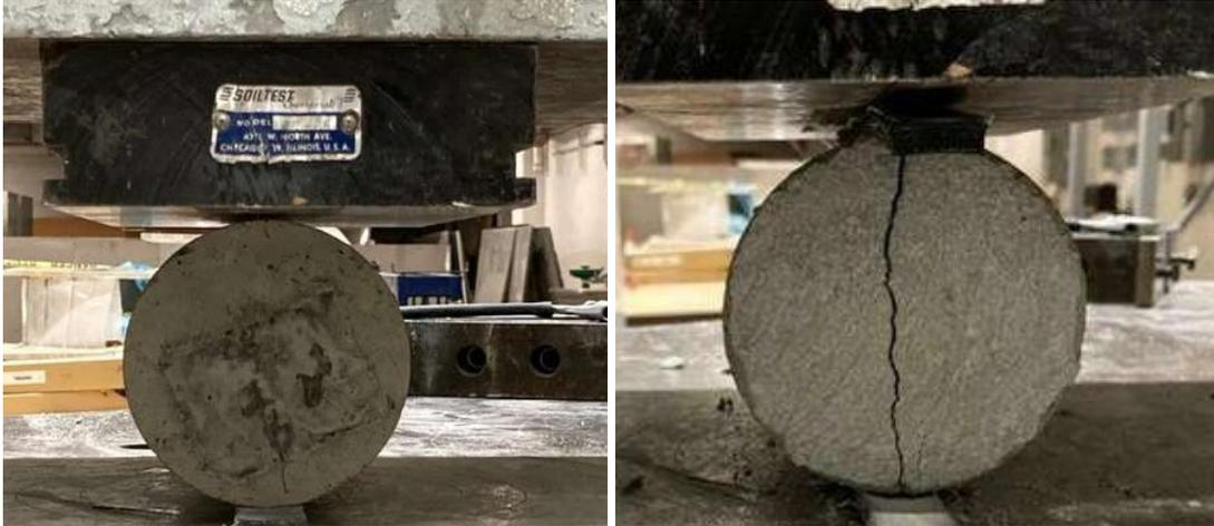
**Figure A.17** Splitting tensile test for the concrete cylinders
