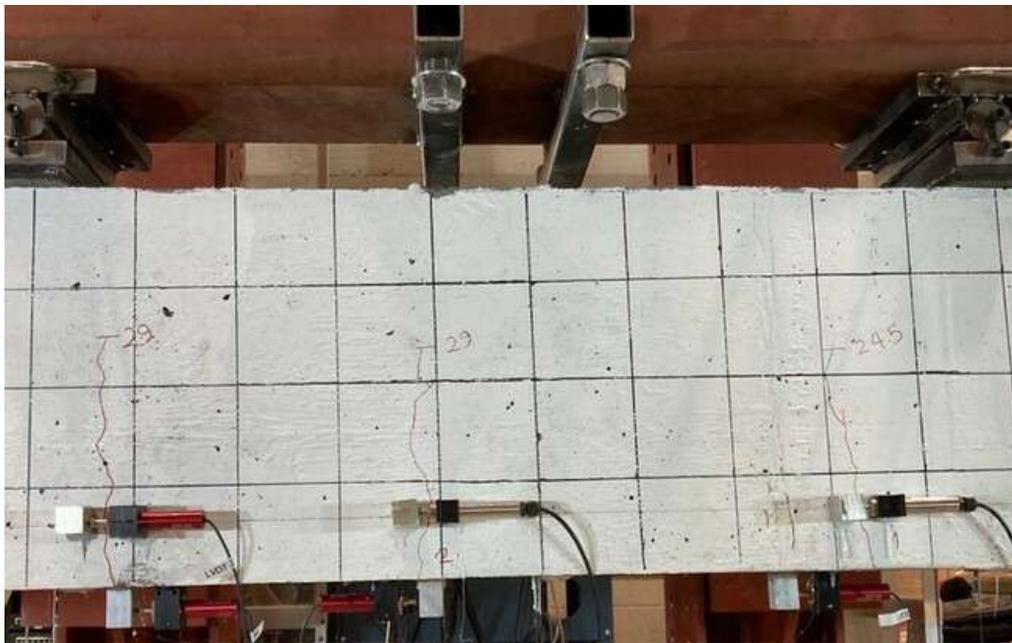
**Figure A.20** Six attached LVDTs at the concrete beam side and bottom faces
