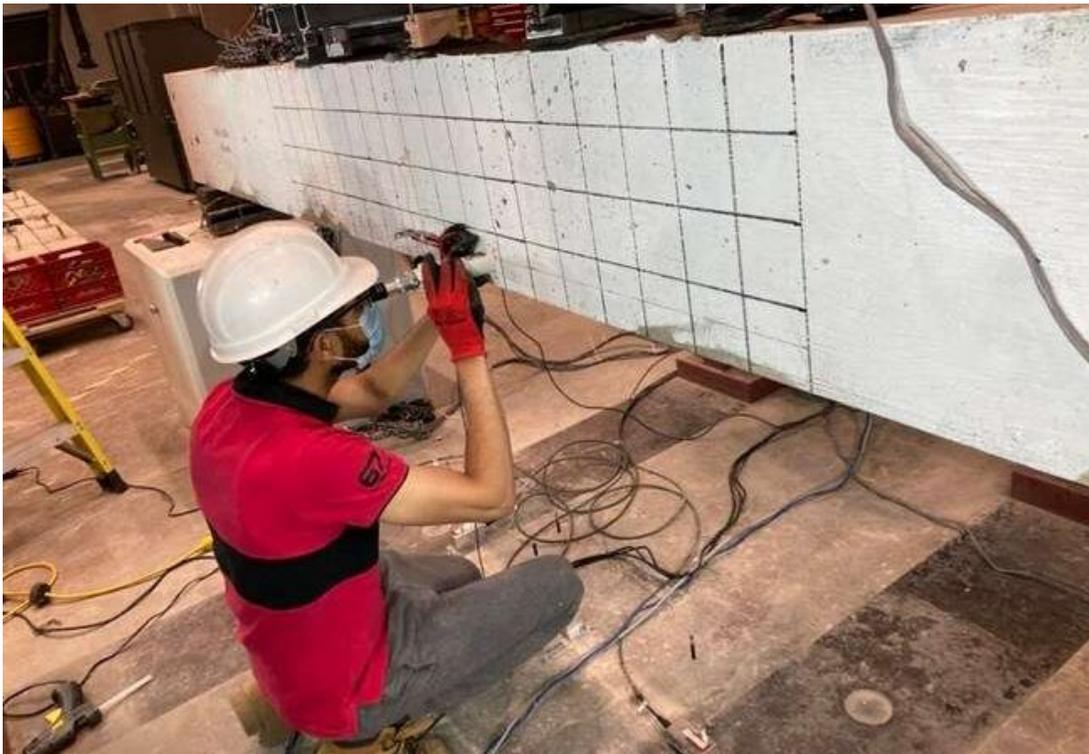
**Figure A.18** Measuring the initial crack width using a hand-held microscope
