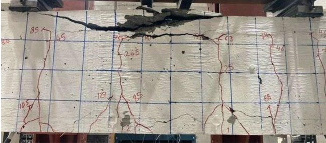
**Figure A.21** Typical concrete compression crushing
