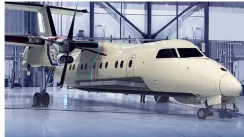
(d) UTC Project 804 [6], [7] is a demonstrator platform using a DHC8-300 regional aircraft for hybrid-electric technologies.
