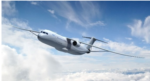
(a) Boeing SUGAR Volt [3], a 150 PAX commercial transport concept with a truce-braced high-wing design.
