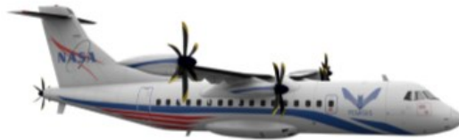
(c) The NASA PEGASUS [5] concept is a 40-50 PAX aircraft based on the ATR42 regional transport.
