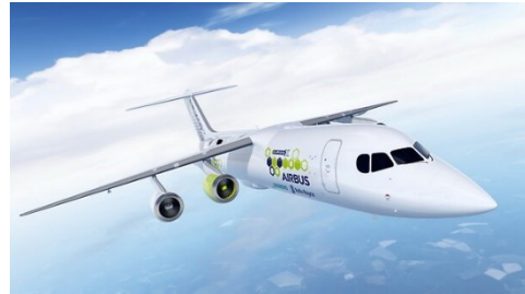
(b) Airbus E-Fan X [4] is a 70 PAX regional transport based on the Bae-146 airframe.
