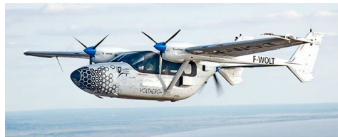
(e) The VoltAero Cassio [8] is a 4-10 PAX prototype hybrid-electric aircraft in the commuter category. It is based on the Cessna 337 airframe and currently undergoing flight testing.
