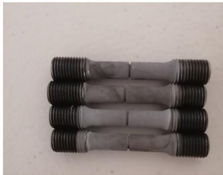
Figure 3-9 Batch of samples plated with Zn-Ni
