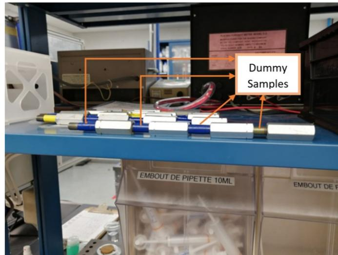
Figure 3-12 Dummy samples used to replace fractured samples in SLT
