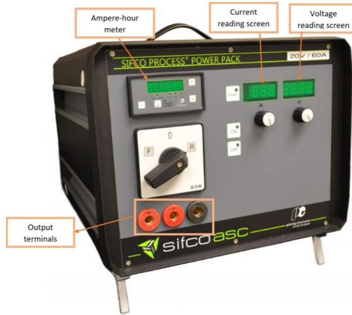
Figure 3-6 Rectifier used for brush plating
