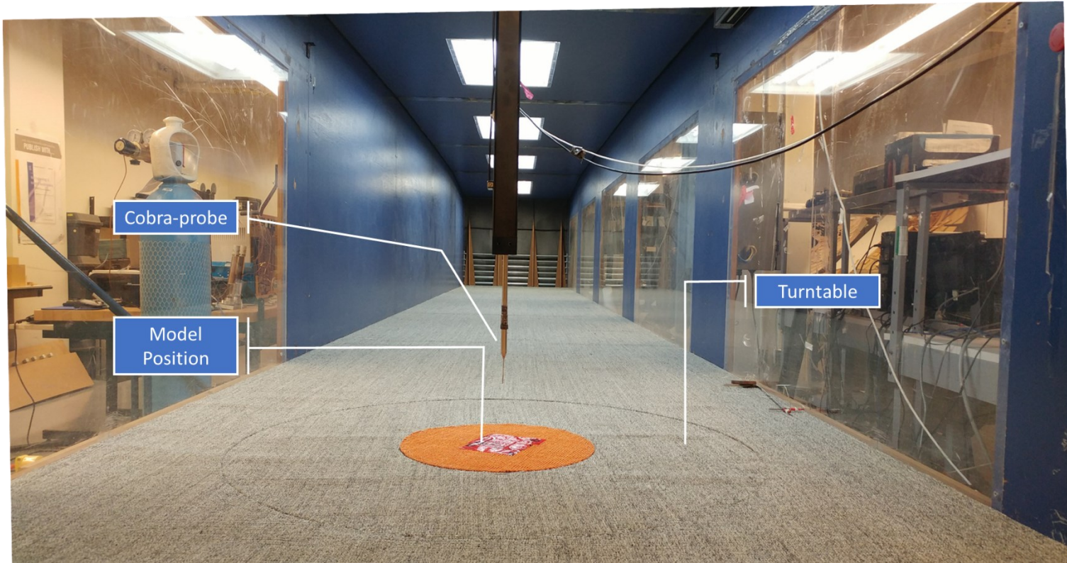
Figure 4.2 Upstream-view photograph of the boundary layer wind tunnel of Concordia University
