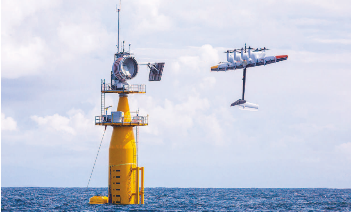
Figure 1.3: Figure showing the drag mode kite Makani M600. The image was reproduced from Ref. [2].
