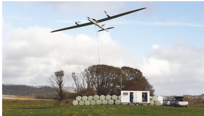
Figure 1.4: Figure showing the lift mode kite from Kitemill. The image was reproduced from Ref. [3].
