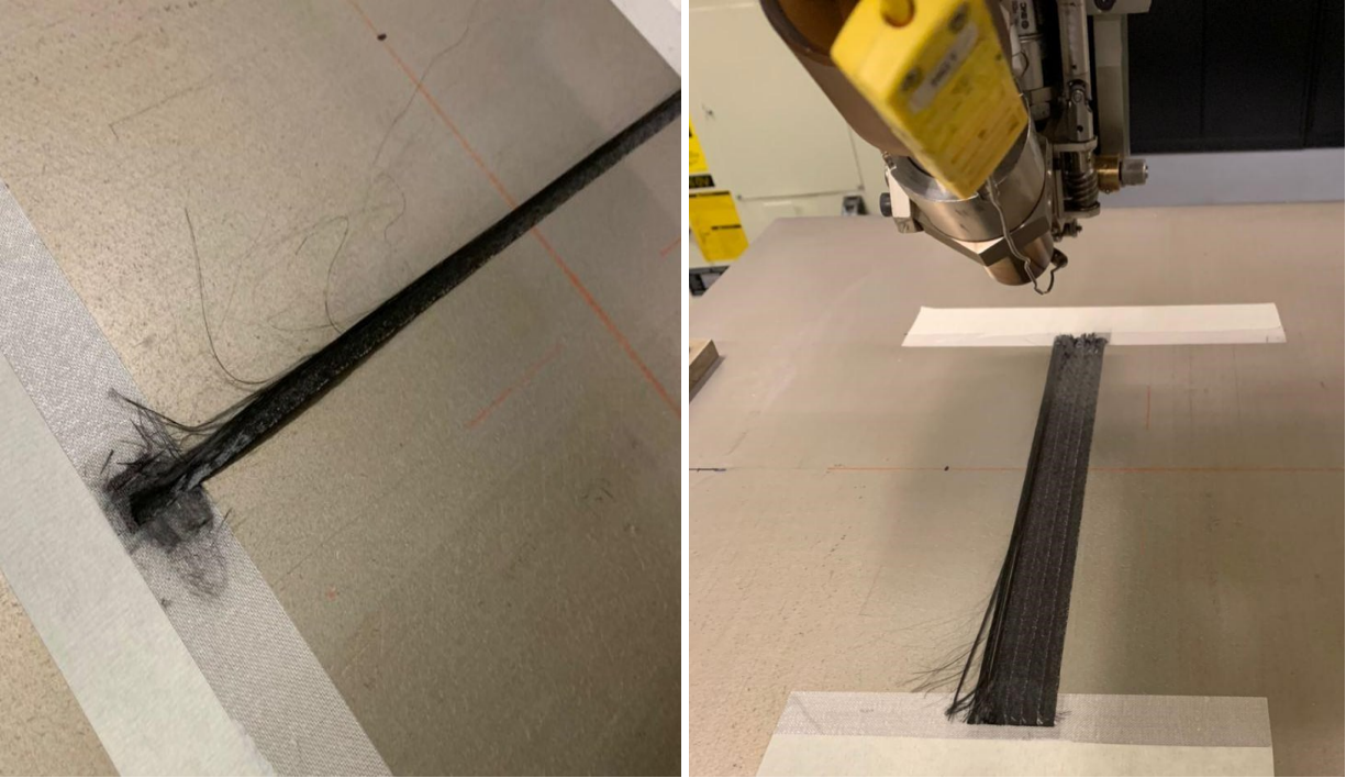
Figure 19. Rolls up in the 2 nd deposited tow
