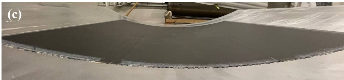
Figure 75. 4 th panel after infusion (a) bag side (b) tool side (c) cross-section
