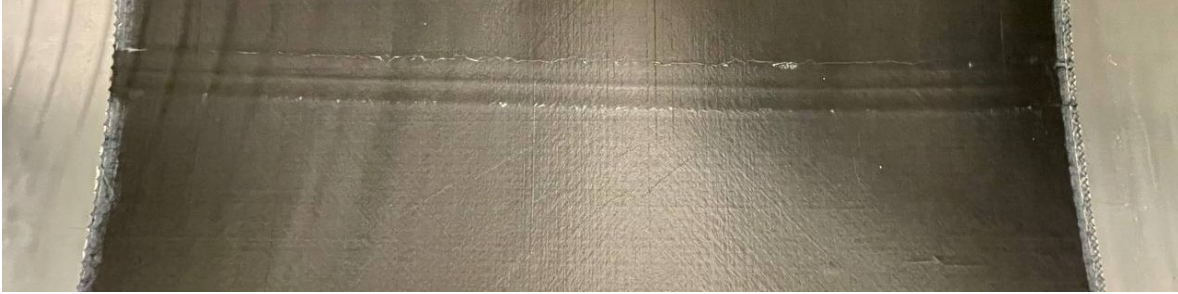
Figure 76. Omega channel imprint on the bag side of the 4 th panel
