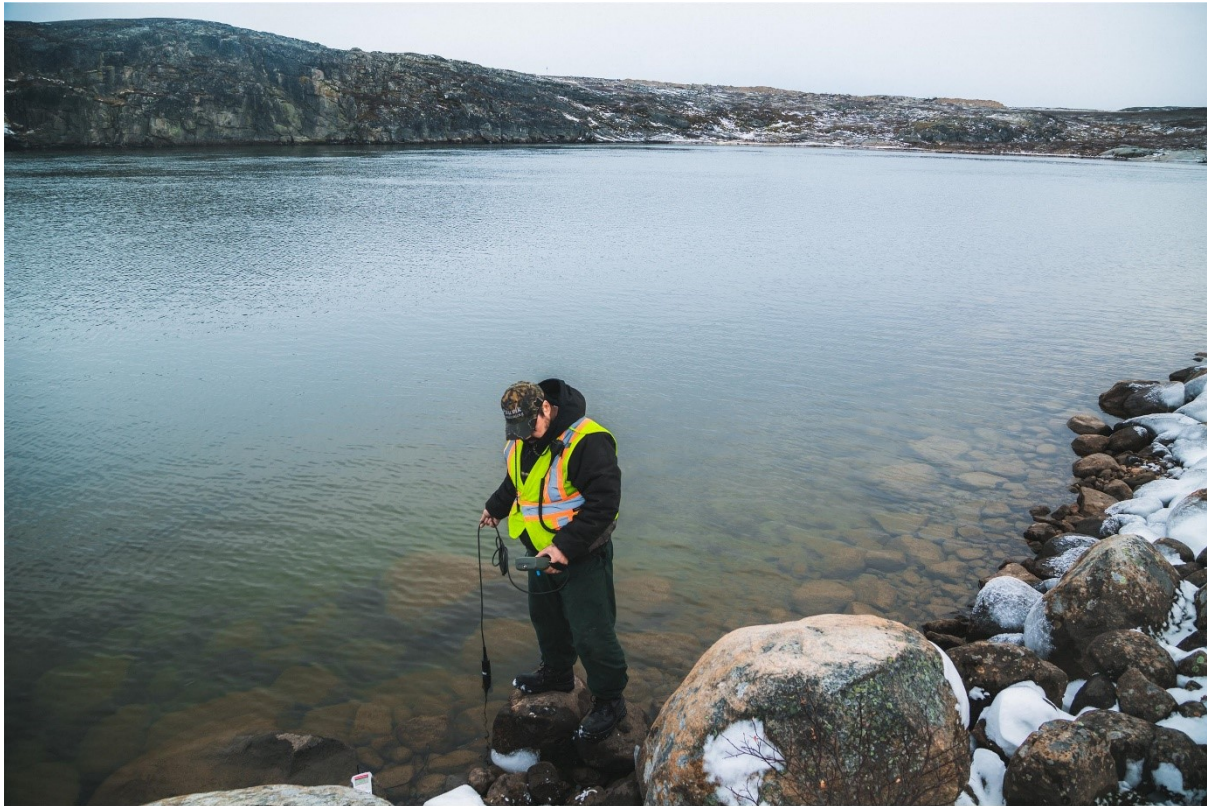
20. Every day, Eric Atagotaaluk tests the water downstream from the construction site. Here he checks the turbidity, temperature and pH of the water. The results of this test showed that the water quality was at normal levels.
