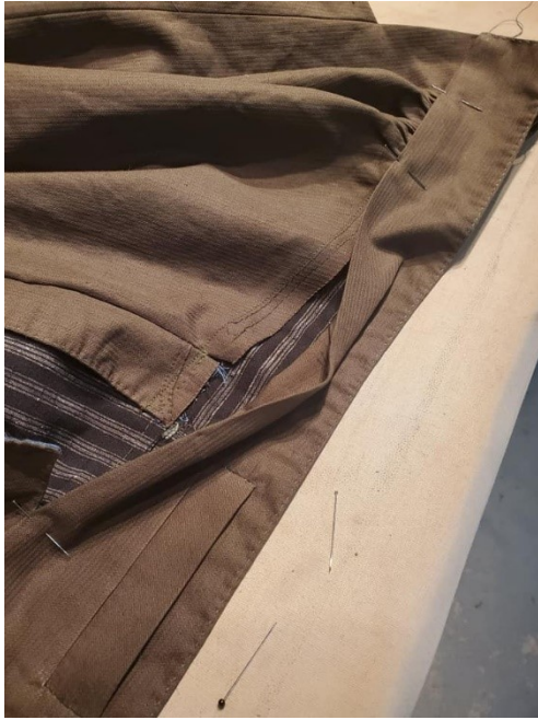
Figure 3-33 Waistband is stitched wrong sides together with the breeches first.
