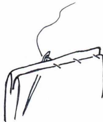
Figure 3-20 Felling: layine, etc Stitch
