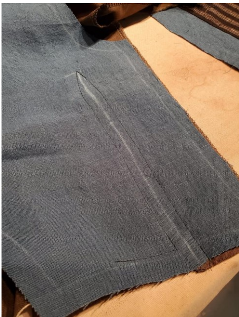
Figure 3-30 The stitching along the top edge of the pocket, and both sides of the deep V of the opening.
