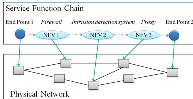
Figure 8: Service Function Chain mapping (Source: Fig.1 in [26])
