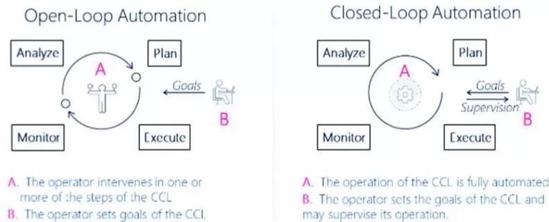
Figure 9: Open-loop automation and Closed-loop automation (Source: Fig.1 in [11])
