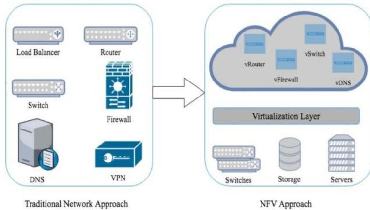
Figure 6: Transformation from traditional network functions to VNFs (Source: Fig.2 in [9])
