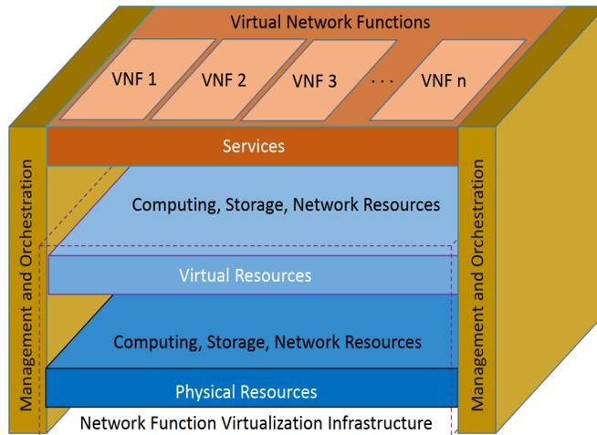
Figure 7: Network Function Virtualization architecture (Source: Fig.4 in [37])
