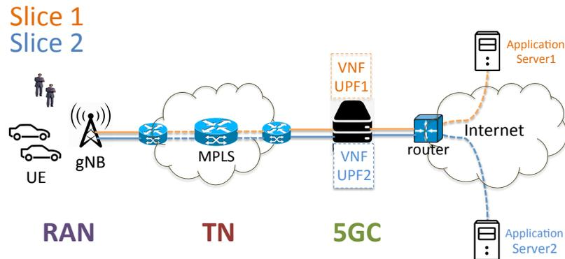
Figure 10: 5G Network slicing simulation model (user plane). Source: Figure 1 in [20]
