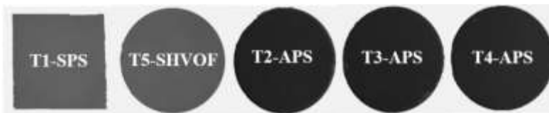
Figure 7.14 The color difference between \text{TiO}_2 coatings produced by various thermal spray processes.
