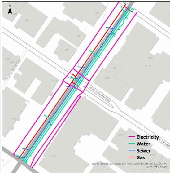
Figure 6-7. Utilities under street segment.
