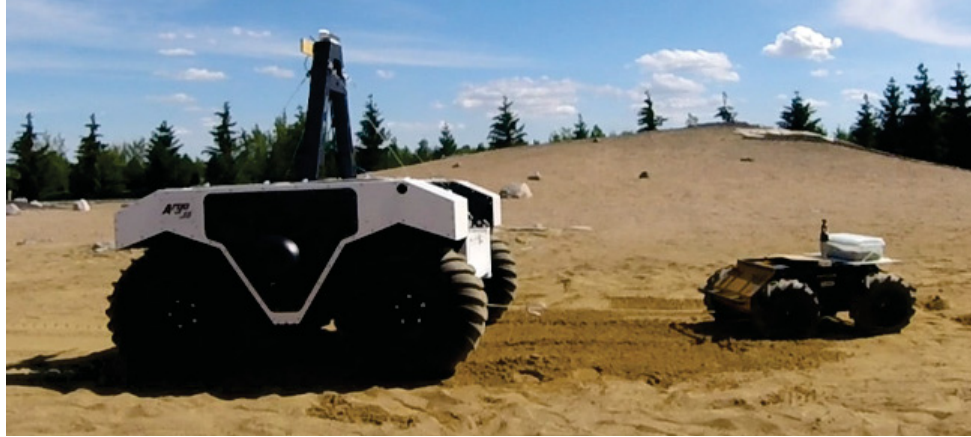
Figure 4.4: Induced slip test setup, with the large Argo J5 rover restricting the Husky rover using a rope.
