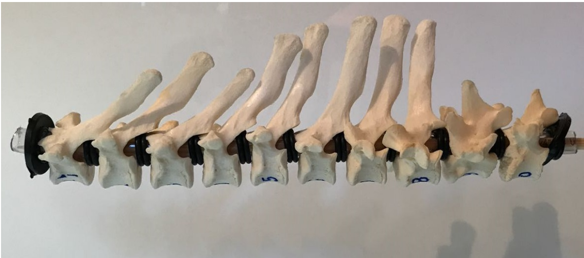
Figure 3.1: Canine vertebrae, with the vinyl tubing inserted through the cavities and the rubber O-rings between each vertebrae, prior to complete immersion into the gel.
