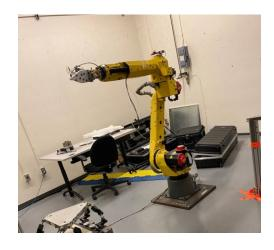
Figure 1-10 Fanuc M20-iA Serial Manipulator
