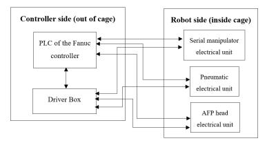
Figure 3-28 Schematic of connections
