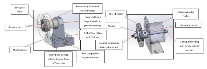
Figure 3-5 Tensioning system design[9]
