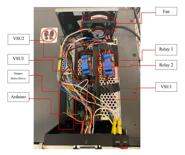
Figure 3-31 Driver box top view and components
