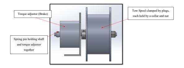
Figure 3-3 Tensioning system on the main spool [9]
