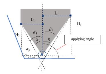
Figure 4-10 The AFP and the part side view with the roller
