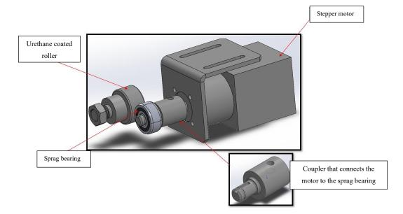
Figure 3-7 Feeding system design[9]
