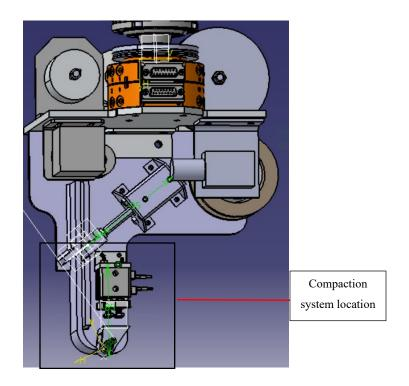
Figure 3-11 Compaction System location
