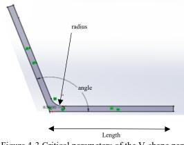
Figure 4-3 Critical parameters of the V-shape part
