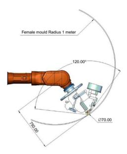
Figure 1-8 Schematic of ADFP (Automated Dry Fiber Placement) deposition head[12]
