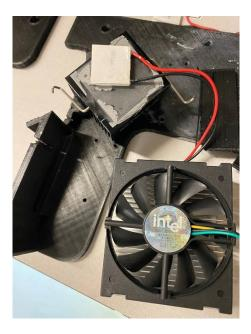
Figure 3-19 Peltier, Fan, and heat sink
