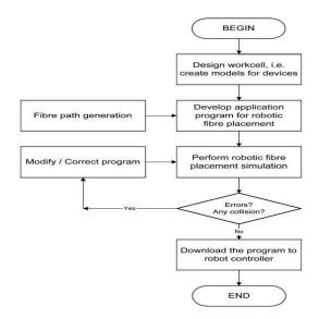
Figure 2-6 Algorithm for off-line programming of robotic fiber placement operation[43]
