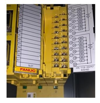
Figure 3-29 Fanuc Modular Output Module[9]
