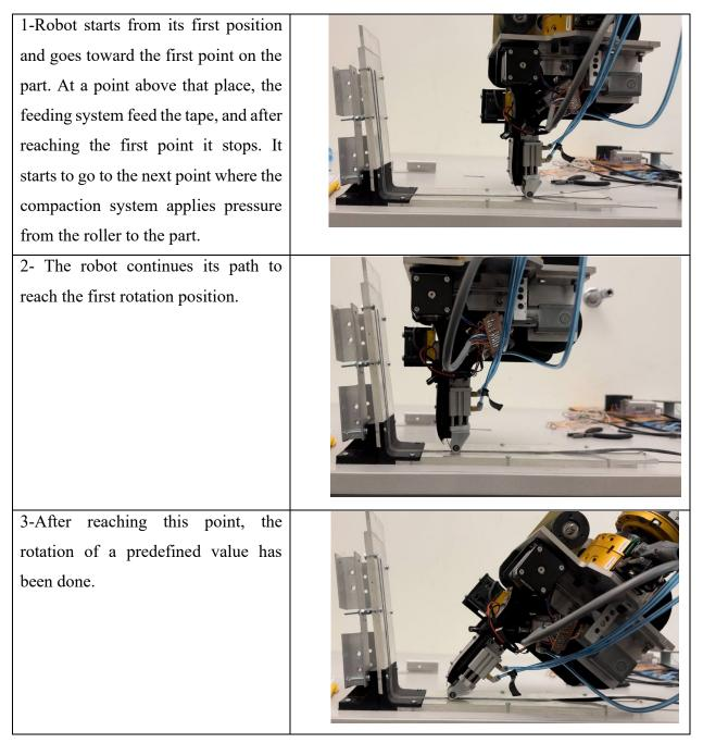
4-The robot continues its path to reach the middle point of the curve of the part which is basically the second rotation point.
