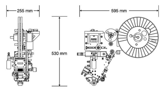
Figure 3-27 Side view and front view of Concordia University AFP head
