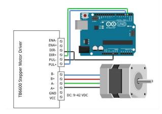
Figure 3-36 Connection of TB6600 to Arduino and stepper motor[50]
