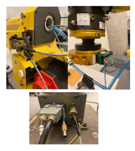
Figure 3-33 Connection of serial manipulator electrical unit
