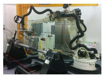
Figure 1-3 A picture of the AFP machine at Concordia University [8]
