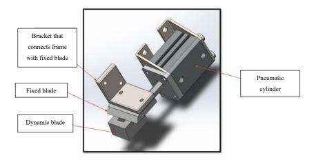
Figure 3-15 Capstone project cutting system design [9]
