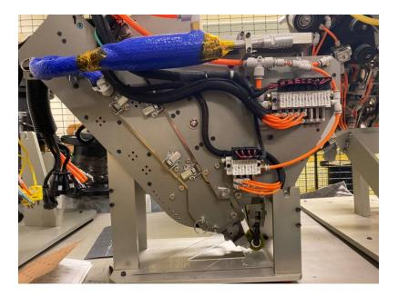
Figure 1-7 Thermoset AFP head at Concordia University
