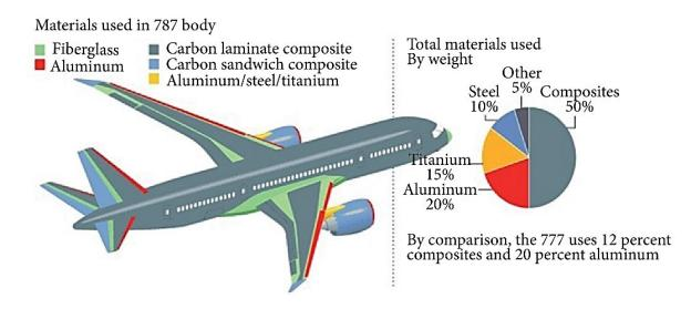
Figure 1-1 Use of advanced composite materials in Boeing 787 Dreamliner [5], [6]
