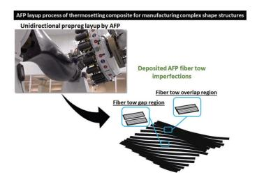
Figure 2-3 Deposited fiber tow imperfections that occur during AFP manufacturing [37]
