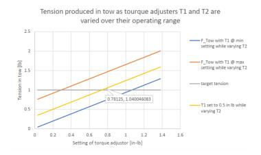
Figure 3-4 Tension produced by Torque Adjustors[9]
