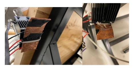
Figure 3-22 Condensation on the Copper plates
