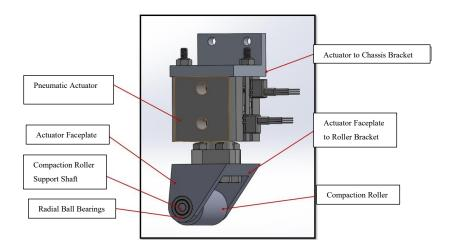
Figure 3-12 Compaction system[9]
