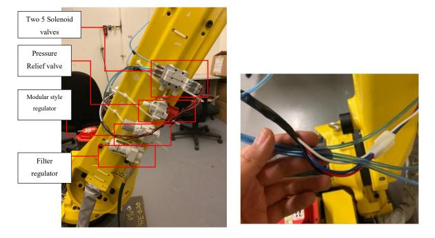
Figure 3-34 Pneumatics systems electrical unit
