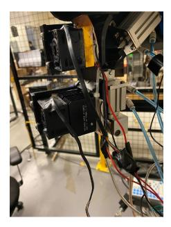
Figure 3-23 Implementing Copper Plates and Peltiers in the proposed project Design
