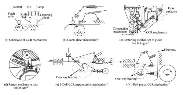
Figure 2-1 Typical CCR mechanisms[14]
