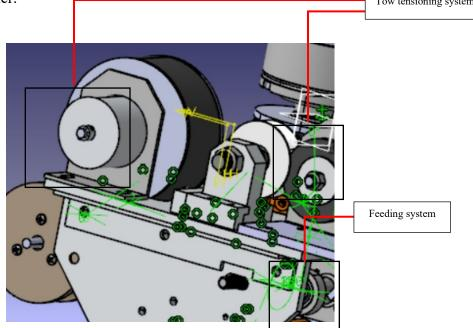
Figure 3-1 Tow tensioning systems and feeding system position on the AFP
