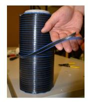
Figure 1-9 1<sup>1</sup>/<sub>4</sub>" width thermoset tow
