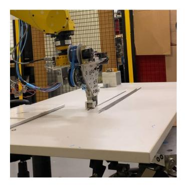
Figure 5-2 Test setup for Automated Fiber Placement on the flat surface
