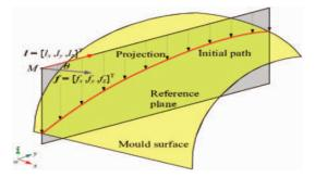
Figure 2-7 Diagram of the fixed angel path planning[44]
