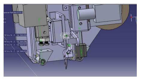
Figure 6-3 AFP head with 2 compaction systems
