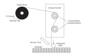
Figure 2-5 Fiber Placement head assembly[40]
