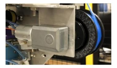
Figure 3-14 DC motor coupled to a spool of collecting system[9]
