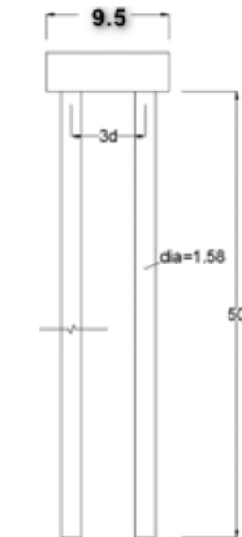
Fig. 3.7-fMPR.1 (dimensions in cm) – Model B (Spacing=3D)
