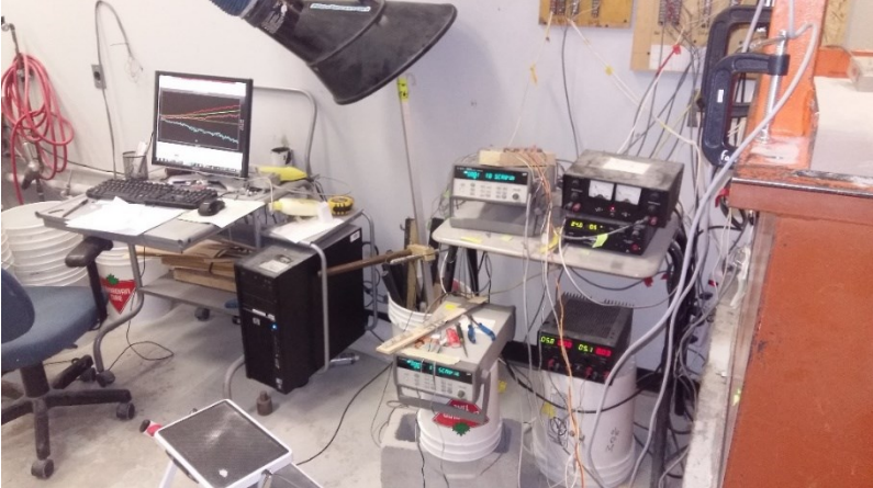
Fig. 4.18- Two DAQs and three power supplies were used to conduct the measurements
