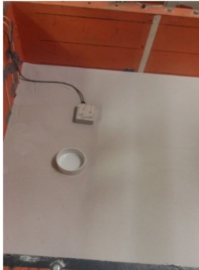
Fig. 3.13-Placing density can and pressure sensors
