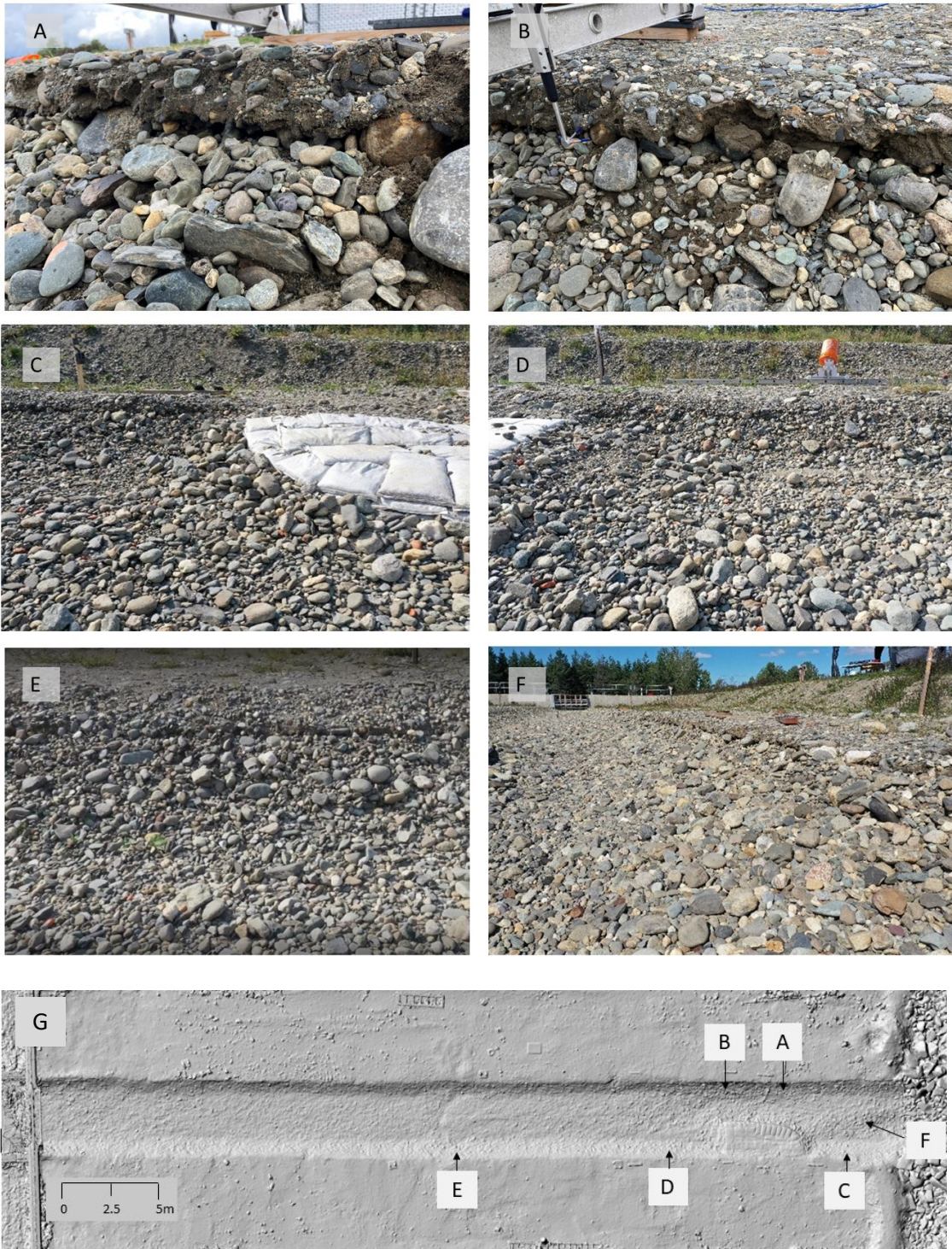
Figure 22: Photograph of the drained river after phase 3. A) upper right bank opposite the perturbation showing visible erosion, B) lower right bank opposite the perturbation showing visible erosion, C) the left riverbank just above the perturbation, and D) the left riverbank just below the perturbation, while E) the midstream left bank (22.5 m), and f) the entire right bank shown from upstream. G) Map represents locations photographs were taken.
