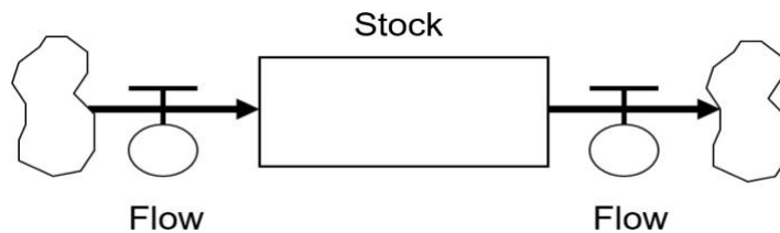
Figure 12. Minimal stock and flow diagram (SFD). The figure comes from (Schoenenberger et al., 2021).
