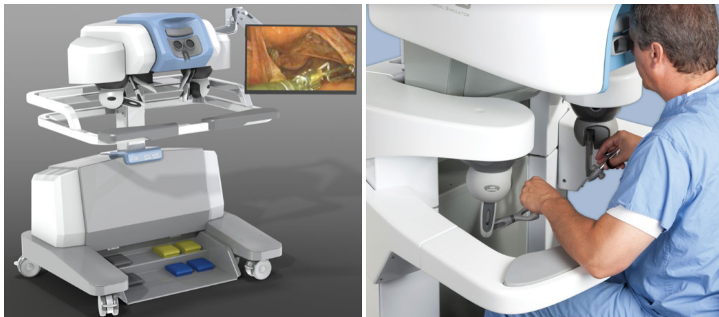
Figure 2.4: RoSS is a robotic surgery simulator with haptic feedback that offers an immersive experience with full-length surgical procedures in 3D [36].
