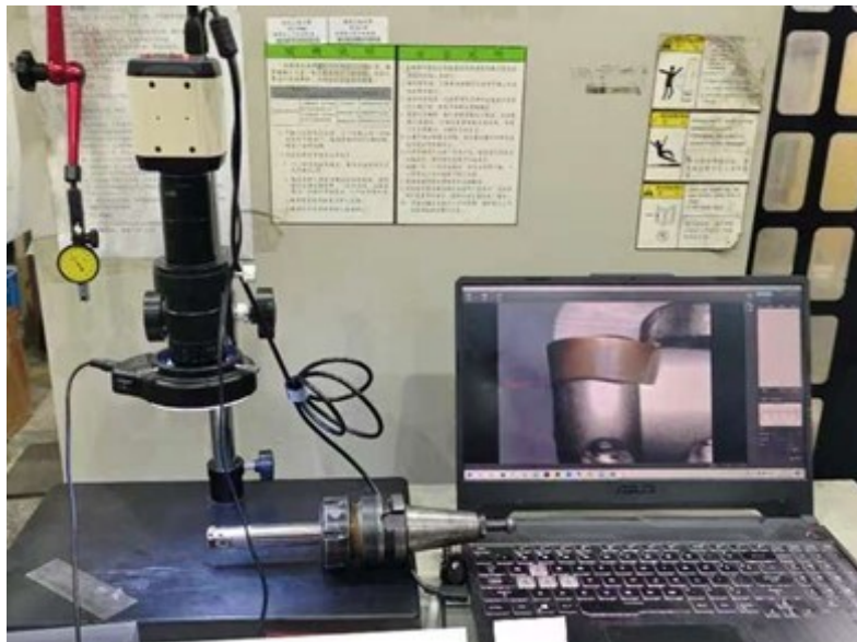
Figure 4.6 The tool wear is observed under the microscope.
