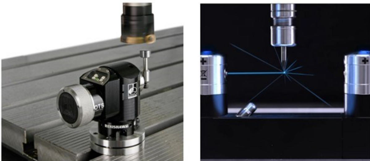
Figure 1.1 A touch probe tool setter and a laser tool setter are shown.
