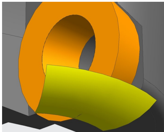
Figure 2.7 The original rotation surface of the round insert is formed.
