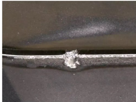
Figure 1.4 Chipping on the cutting edge of the cutting tool.
