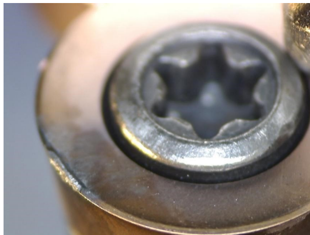
Figure 4.16 The build-up edge is found in the fifth measurement.
