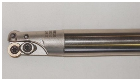
Figure 4.3 The EMR5R two inserts round mill is selected for milling.
