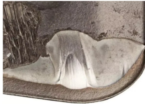
Figure 1.2 Crater wear on the rake face of the cutting tool.
