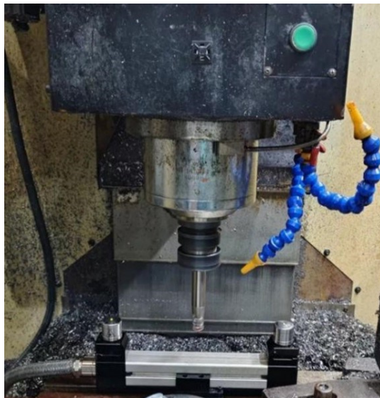
Figure 4.4 The round inset tool is measured by the OMM system.
