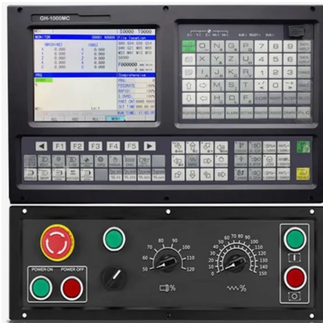
Figure 1.16 The CNC controller processes the signal sent from the interface.
