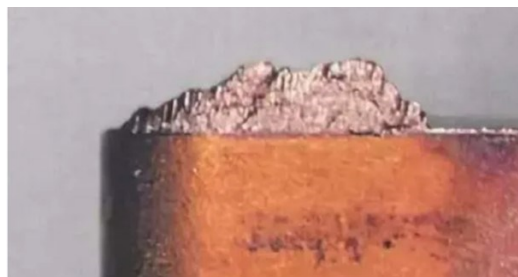
Figure 1.3 Build-up edge adheres to the cutting tool.
