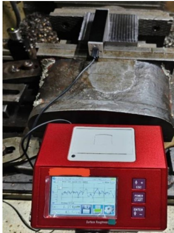
Figure 4.15 The surface roughness is measured after milling each 1mm layer of the workpiece.
