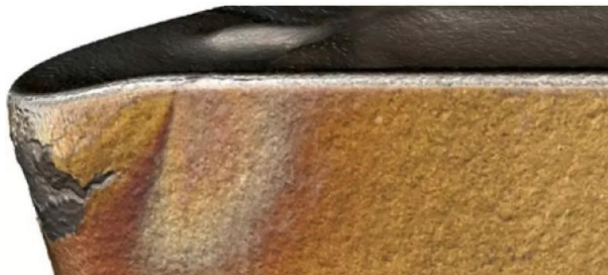
Figure 1.6 The cutting tool is softened due to temperature.
