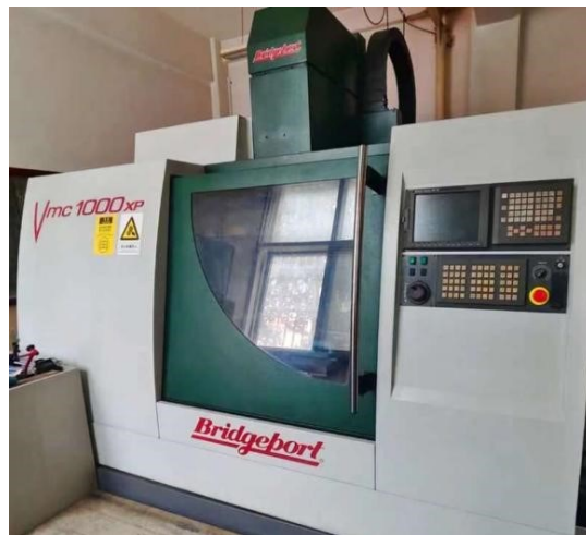
Figure 4.2 The Bridgeport VMC 1000xp 3-axis CNC machine is selected for milling.
