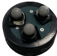
Figure 4.1: The Vicon-specific markers attached to the hockey puck.
