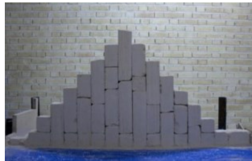
Figure 5-4: (a) A sketch of the geometry, and (b) the physical model for the randomly arranged blocks (Amini et al. 2015)
