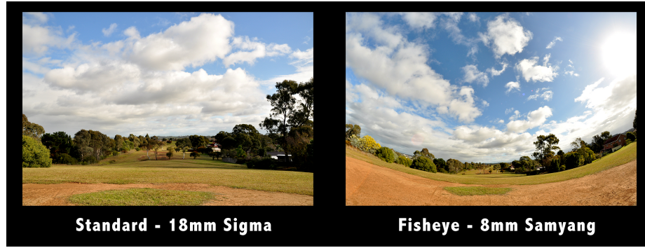
Figure 2.1: Same scene captured by a standard and a fisheye lens. Source: [1]
