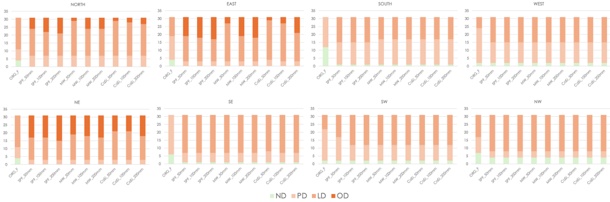
FIG – C6. The predicted mechanical FT damage for pre- and post-retrofit masonry walls – F_E=1.4 and F_D=0.5 ; F_E=0.7 and F_D=1.0 .
