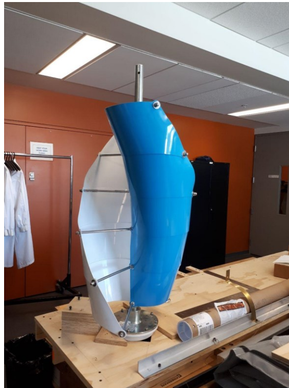
Figure 85- Final assembly of RX-SV2 wind turbine.
