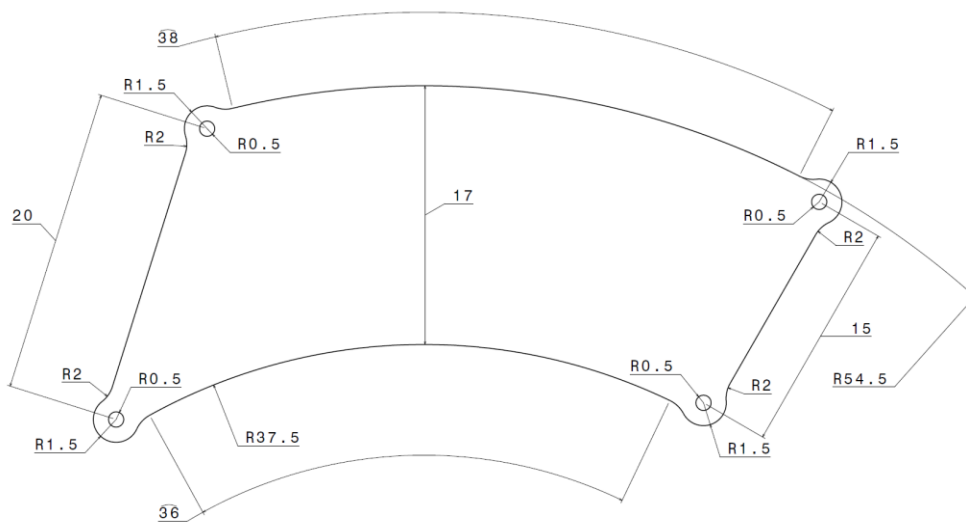
Figure 96- The CAD model of the 2D model of the wind turbine segment, all sized are in cm.
