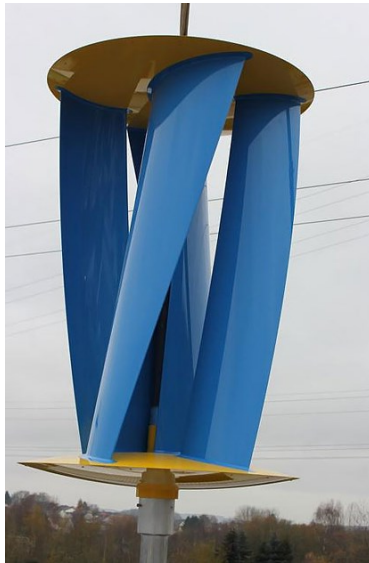
Figure 79- Savonius vertical-axis wind turbine made by Techcarbon company [63].
