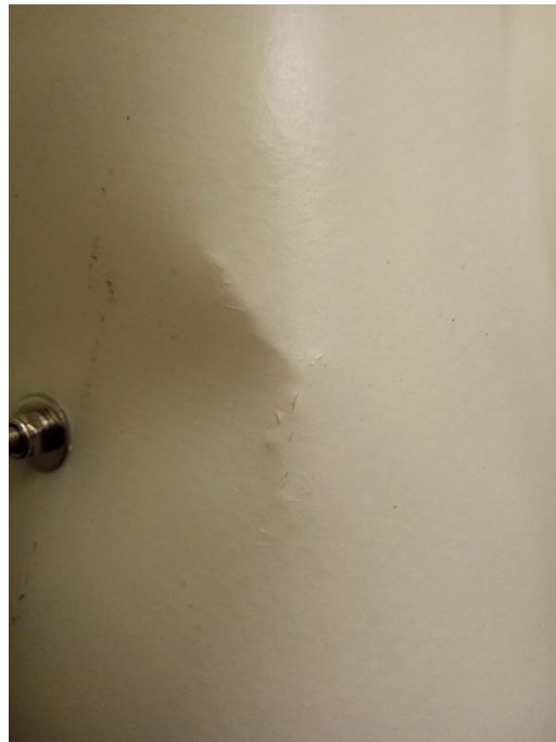
Figure 86- Cracks on the blades of RX-SV1 after final assembly.
