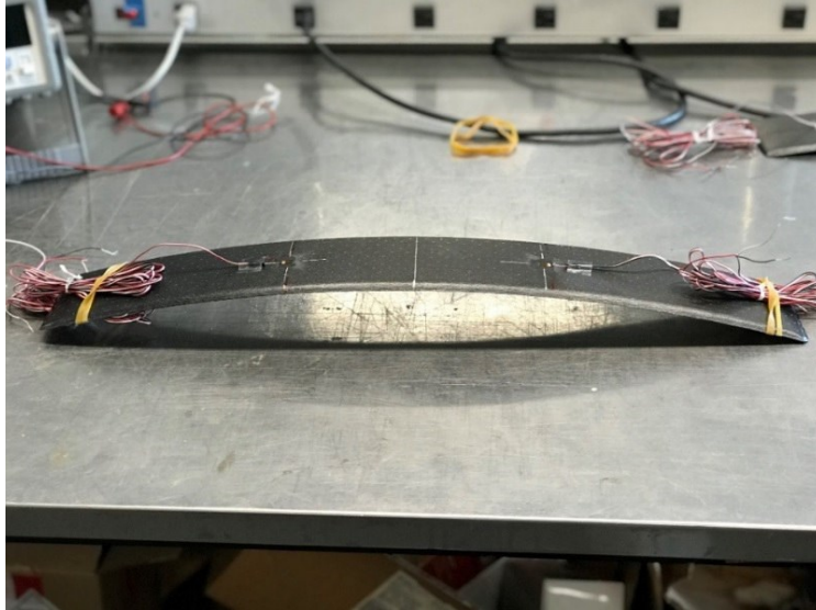
Figure 12- 24-inch long composite leaf spring [14].
