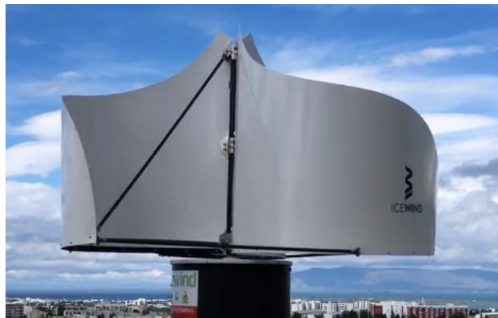
Figure 82- Savonius vertical-axis wind turbine made by ICEWIND [59].
