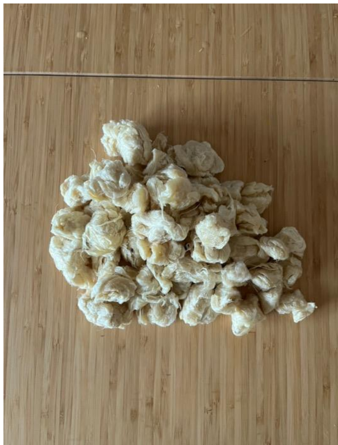
Figure 32. Audet-Arcand, A. (2023). Cooking milkweed fibres.
