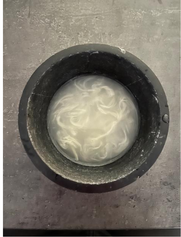
Figure 35. Audet-Arcand, A. (2023). About to hand-grind milkweed fibre with mortar and pestle.
