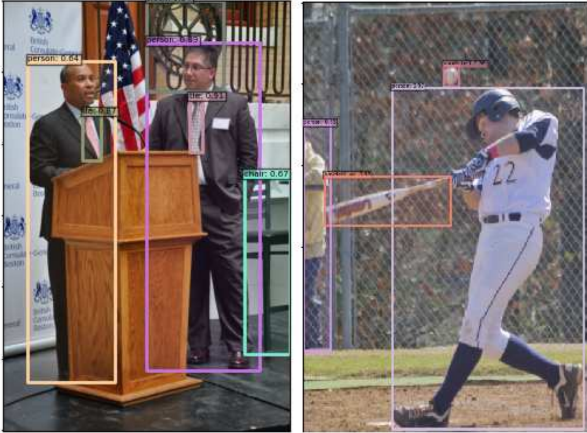
Figure 1.1: Two images with colour-coded bounding boxes labelled with the object category and confidence (conf.) score, illustrating the DINO model’s performance. In the left image, detected objects include Person 1 (conf. 0.64), Person 2 (conf. 0.89), and a Chair (conf. 0.67). In the right image, detected objects include Person (conf. 0.97), Baseball bat (conf. 0.93), and Baseball ball (conf. 0.98).
