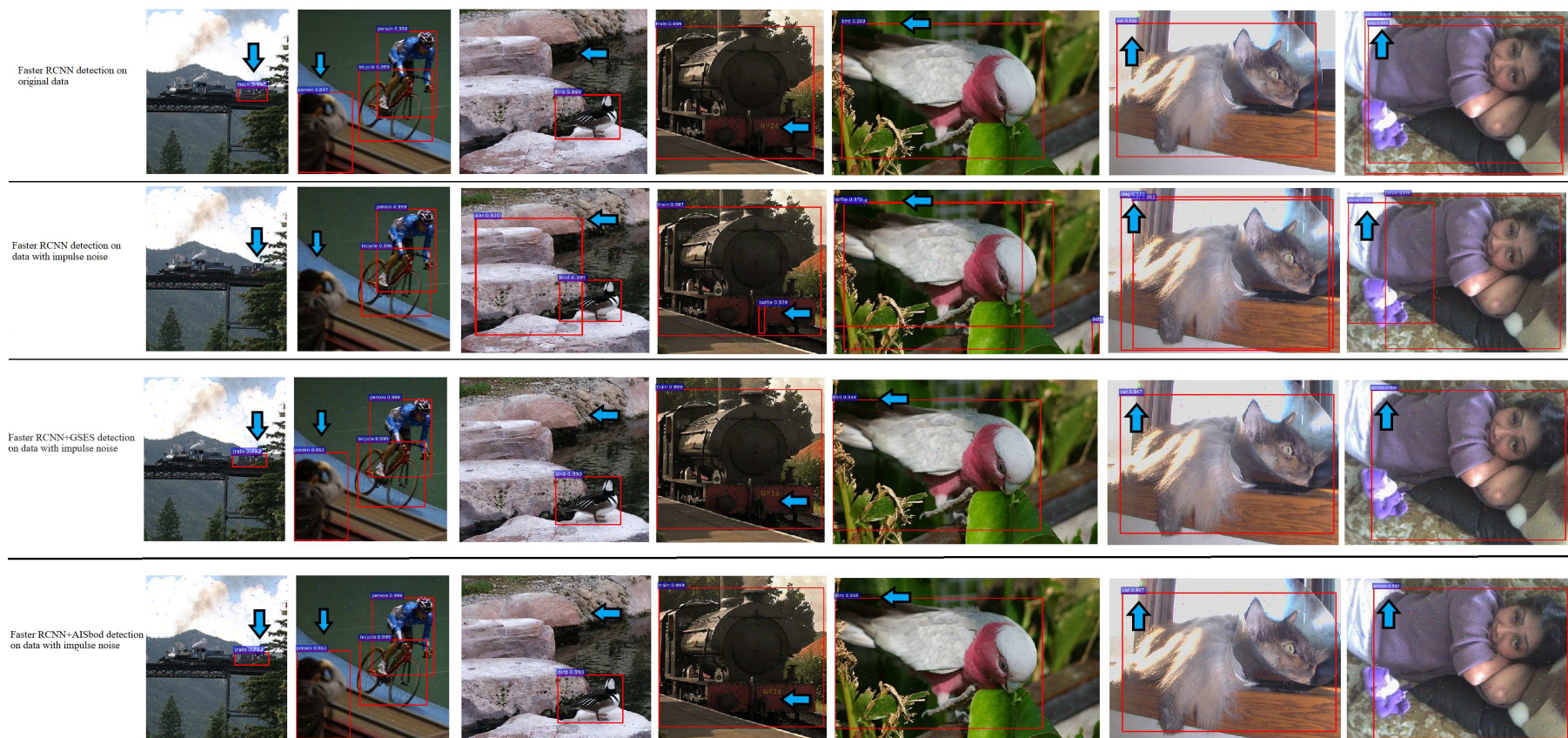
Figure C.2: Comparison of Faster RCNN, Faster RCNN+GSES, and Faster RCNN+AISbod on 0.25% impulse noisy samples. For instance, the Train correctly detected in the original image (row 1, column 1) is missed in the noisy version (row 2, column 1). This error is corrected in GSES and AIS (rows 4 and 5, column 1). (Points of interest indicated by blue arrows are better viewed by zooming in).
