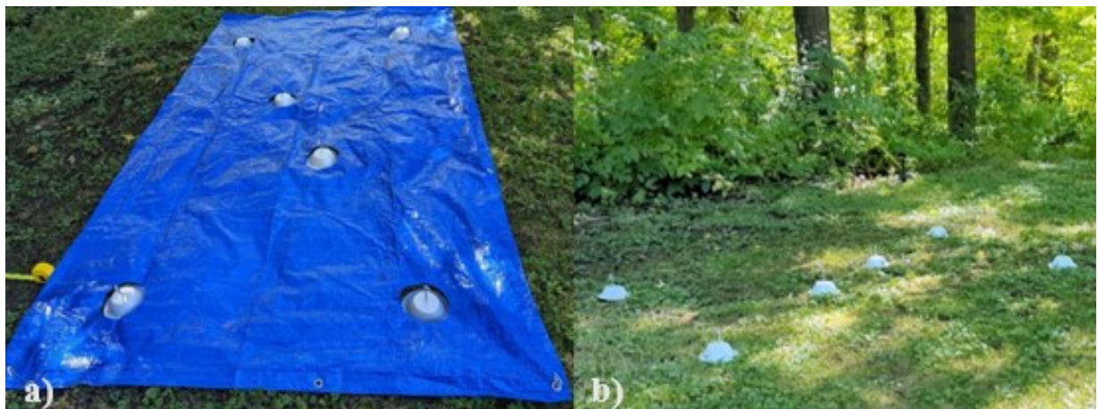
Figure 4: Array setup in the field, a) Initial array setup with tarp template. and b) Fully assembled and operational array.
