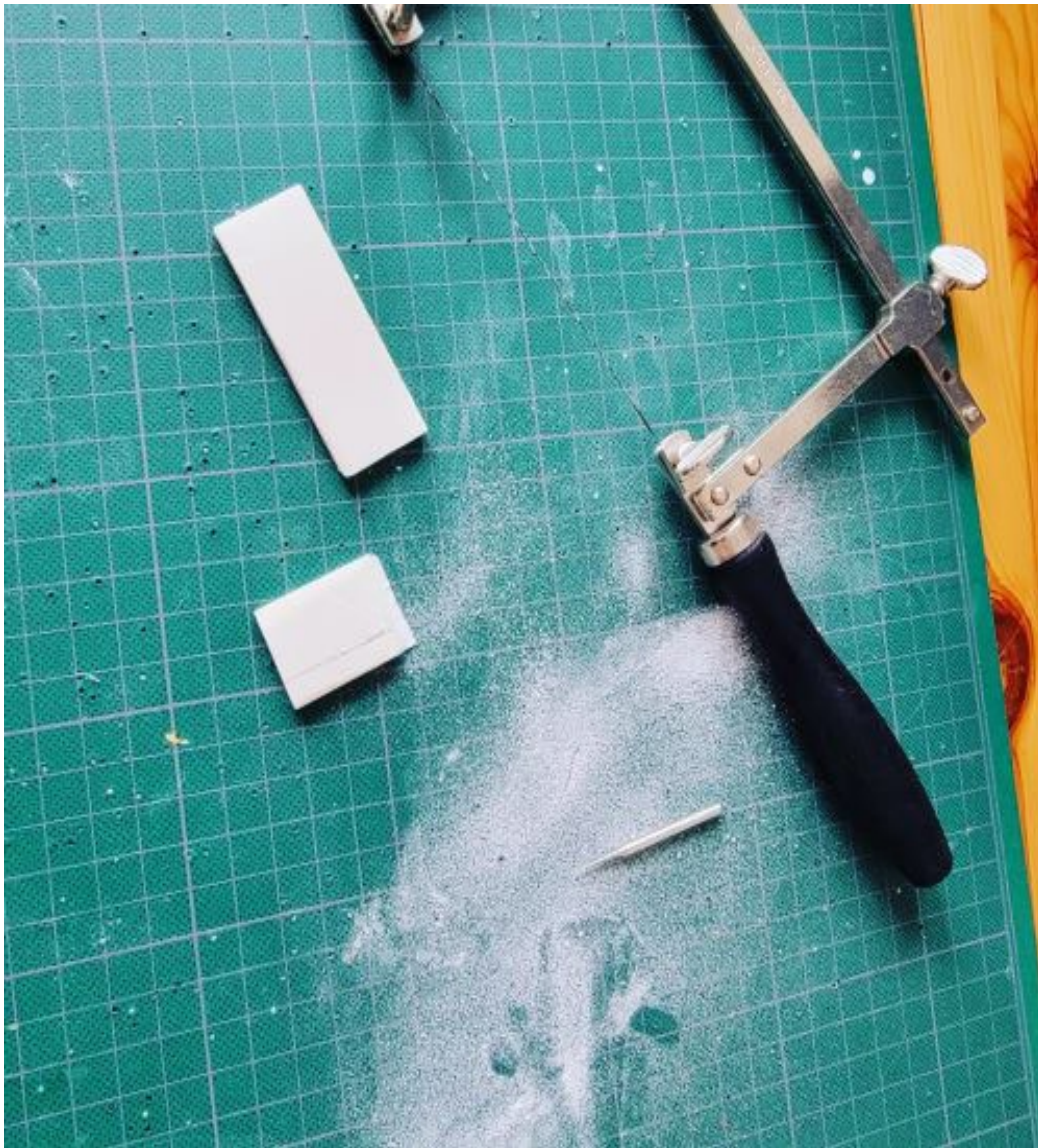
Figure 33: Hand saw, bovine bone pieces to make traditional tattoo tools, Mel Lefebvre and Dion Kaszas, 2021.
