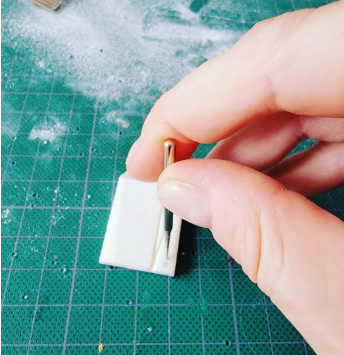
Figure 34: Diamond drill bit, bovine bone piece to make traditional tattoo tools, Mel Lefebvre and Dion Kaszas, 2021.
