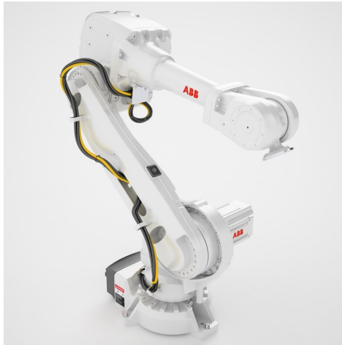
Figure 1-2. Apparatus of six-degree freedom 4600ABB robot (adopted from https://www.turbosquid.com/ko/3d-models/3d-abb-irb-4600-industrial-robot-02-1915018 )
