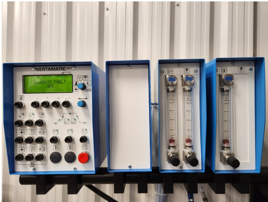
Figure 3-1 Nertamatic plus machine used for welding.
