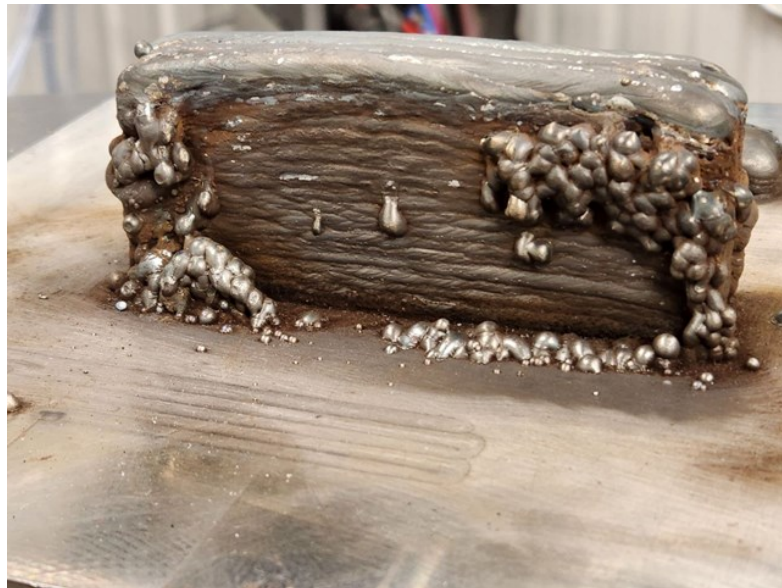
Figure 1-6 Droplet formation during layer deposition
