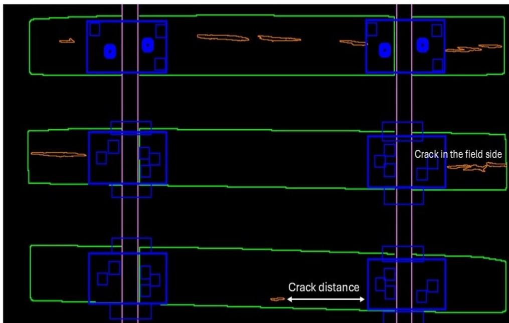
**Figure 7: crack distance from the components.**
