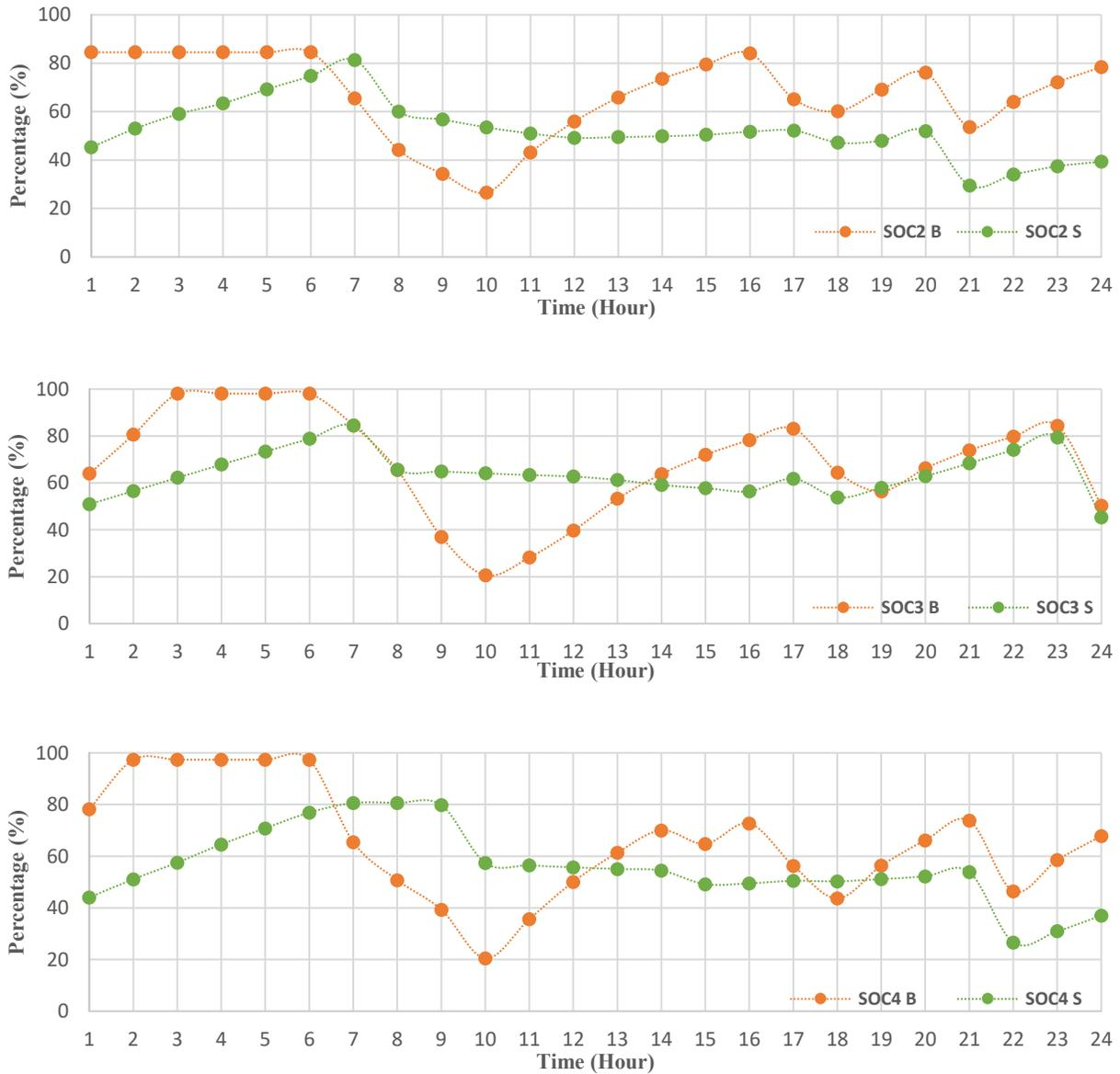
Figure 29. Comparison of SOC of PHEVs in the smart V2G and basic V2G strategies.
