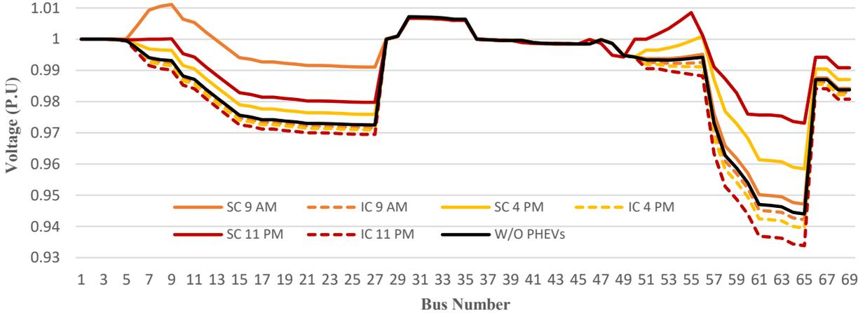
Figure 24. Voltage Profile of the system without PHEVs and with Smart and immediate charging scenarios.
