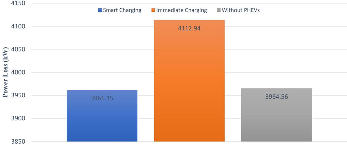
Figure 23. Power losses of the system considering immediate and smart charging network.
