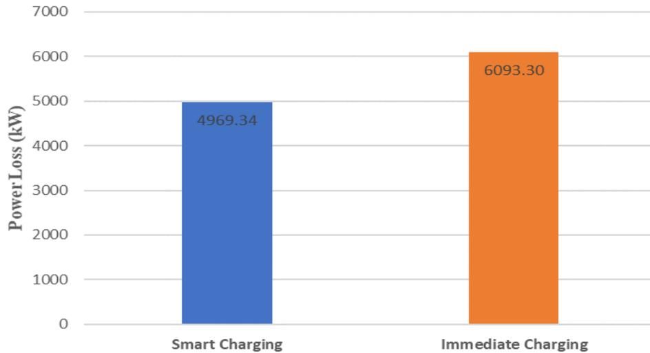
Figure 27. Power losses of the system under the Québec ZEV plan by 2030.
