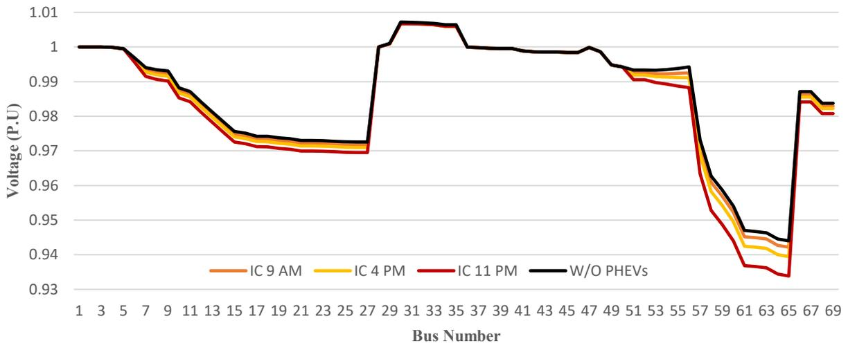
Figure 21. Voltage Profile of the system with and without PHEVs.
