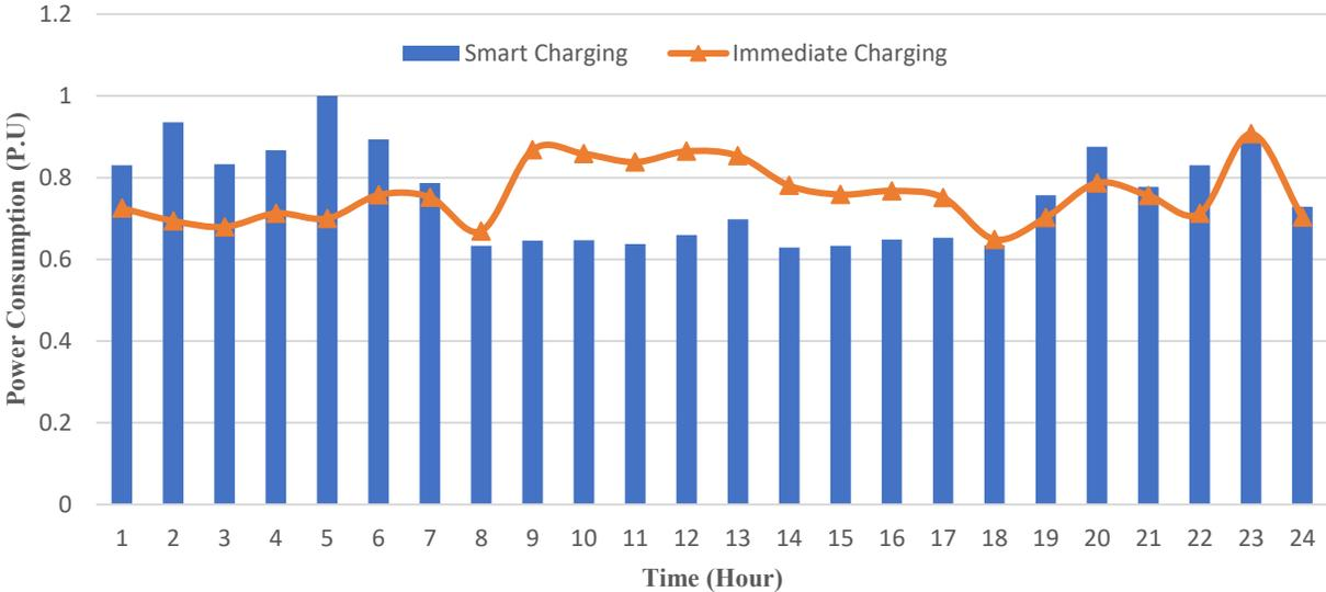
Figure 25. Power Consumption of the network under smart and immediate charging scenarios.
