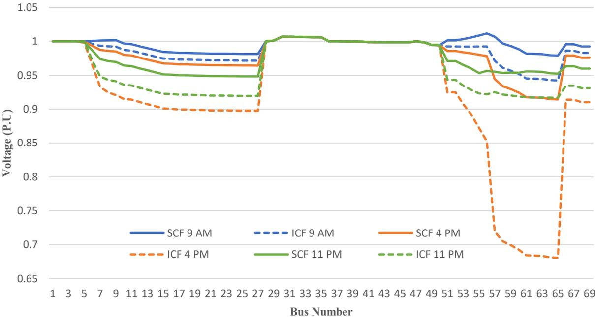
Figure 26. Voltage Profile of the system under the Québec ZEV plan by 2030.
