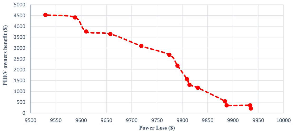
Figure 28. Generated Pareto Frontier using the proposed Epsilon-Constraint method.
