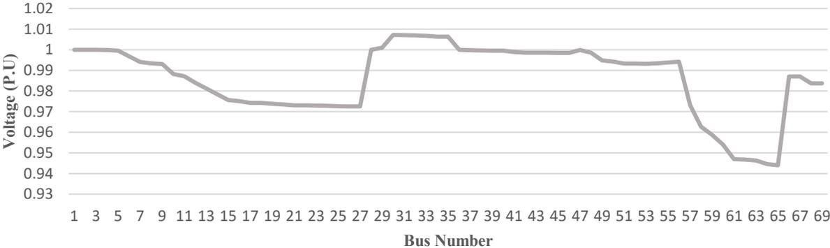
Figure 17. Voltage Profile of the system without the contribution of PHEV.
