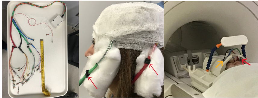
Figure 3.1: Length of the old set of EEG free electrodes (on the left). Metal connectors shown with the red arrows (center). In the coil, eye whole is shown with the yellow arrow and the metal connector inside the coil is pointed with red arrow (on the right) indicating the insufficient length of EEG cables which would cause the connectors remain inside the coil and create artifact on MR Images.
