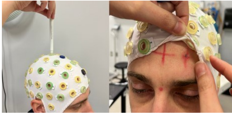
Figure 3.5: Marking the electrode positions using an EEG cap. The cap was aligned with the 10-20 reference points.
