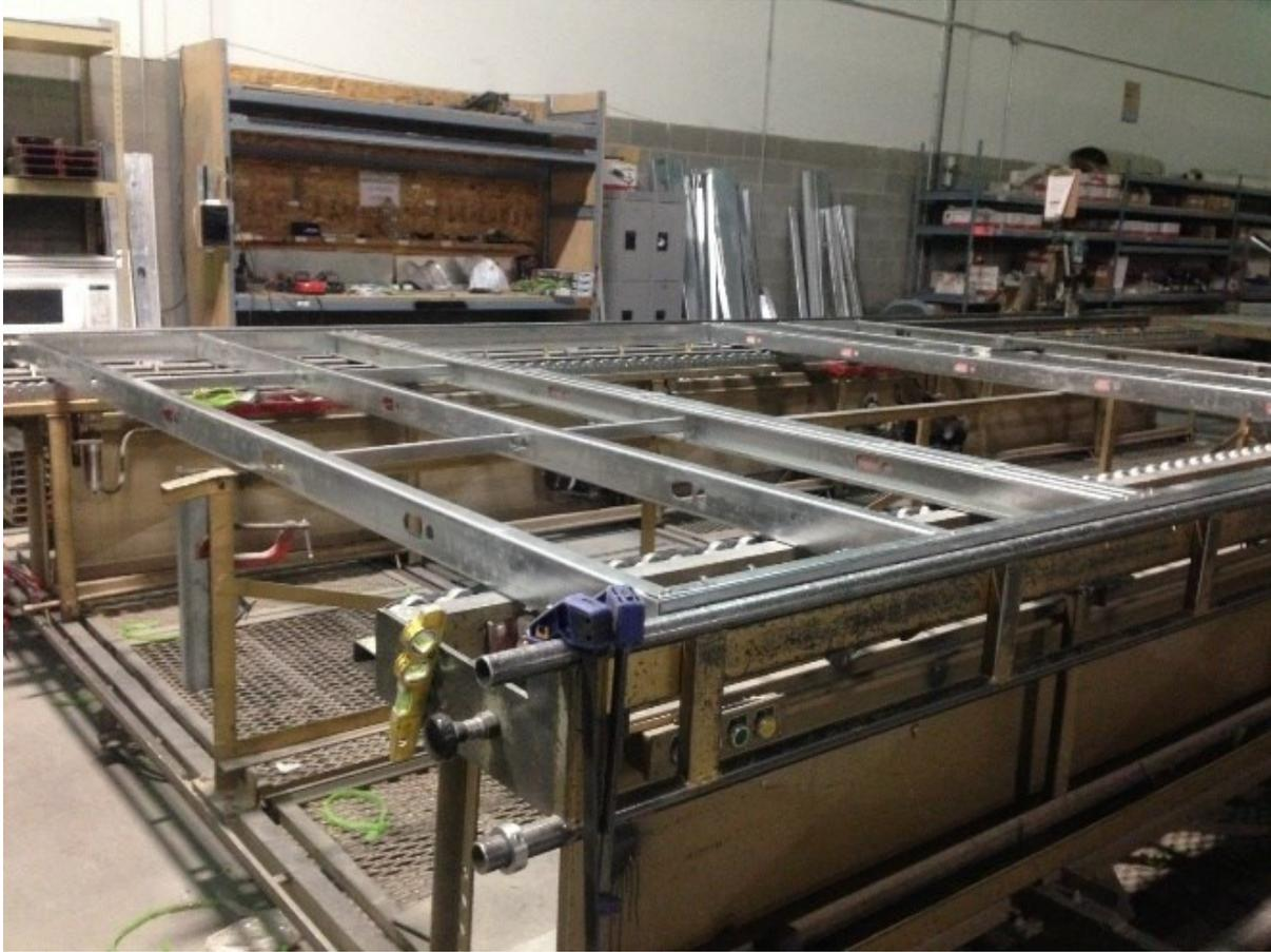
Figure 4.3: Framing workstation
