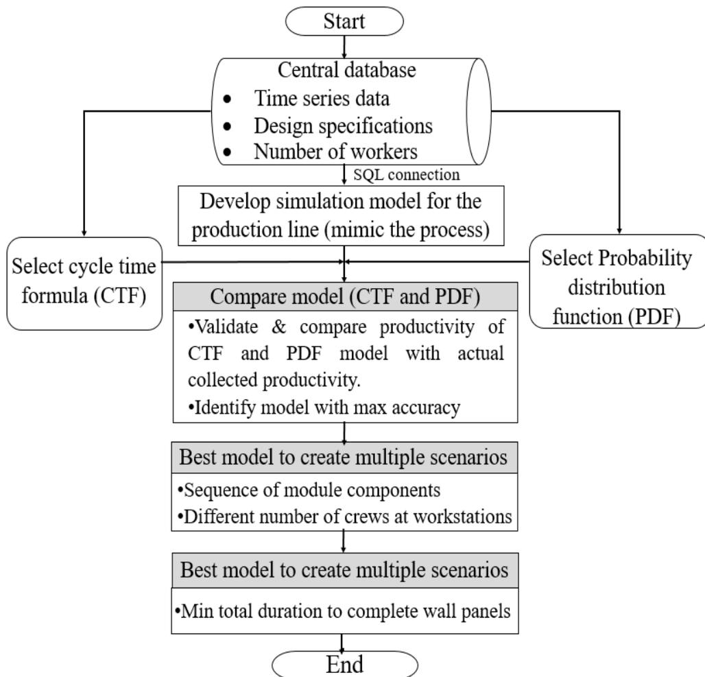
Figure 3.5: Flowchart of simulation-based planning
