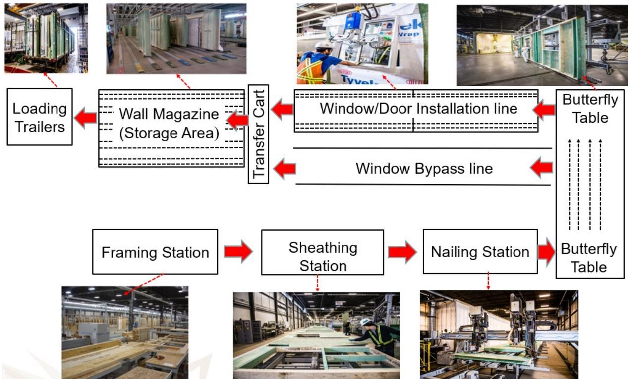
Figure 4.10: Wood-based wall panel production line
