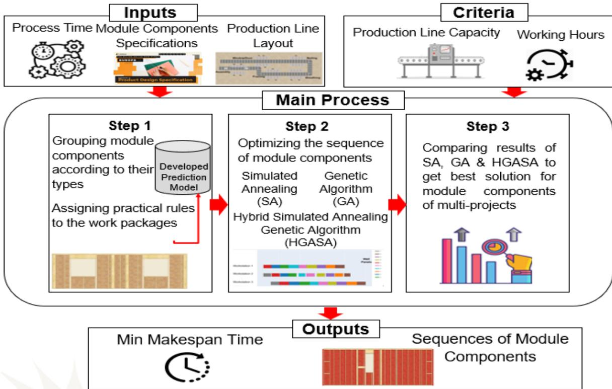
Figure 3.10: Developed method for optimized planning and scheduling
