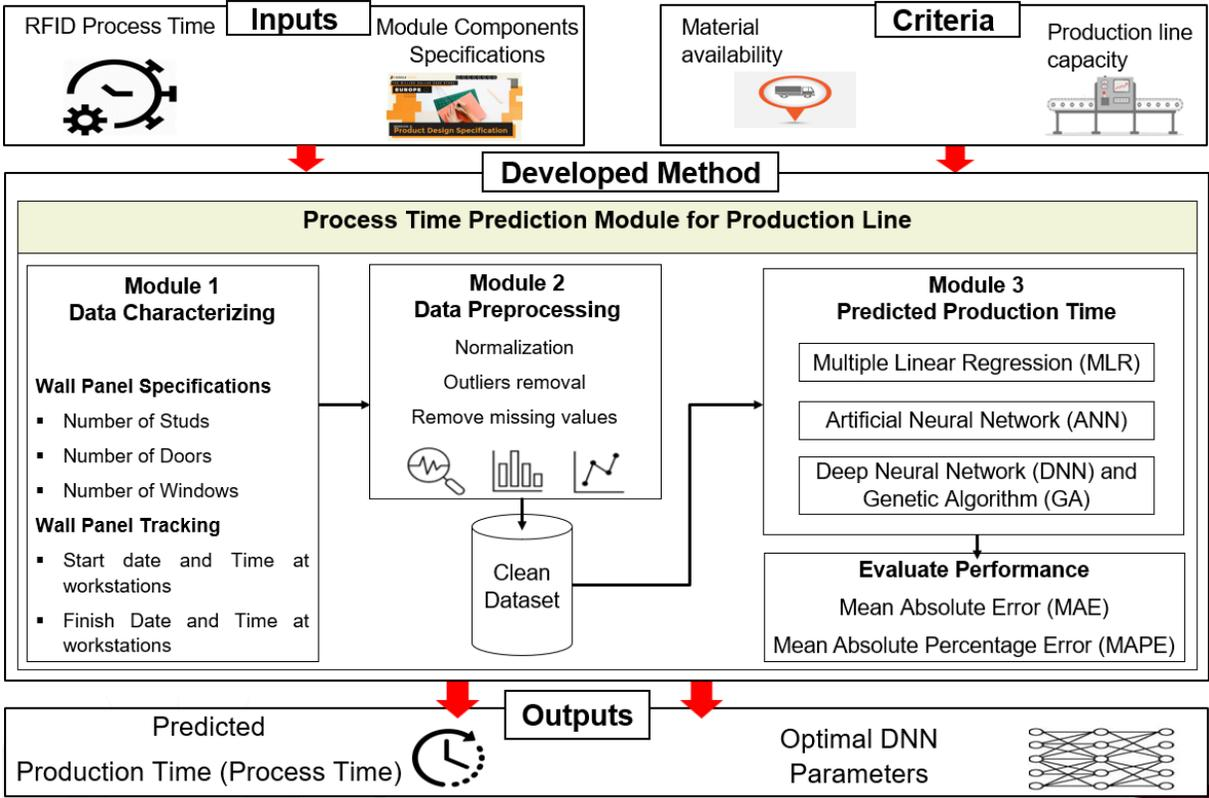
Figure 3.6: Overview of the Developed Method
