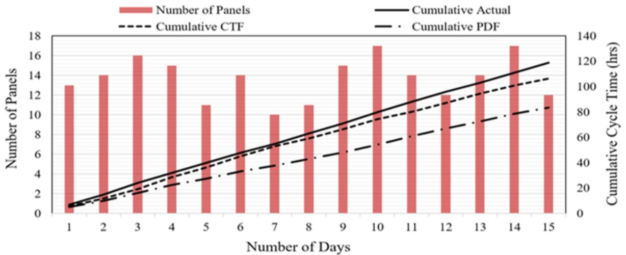
Figure 4.9: Comparison between cumulative actual and simulated cycle time
