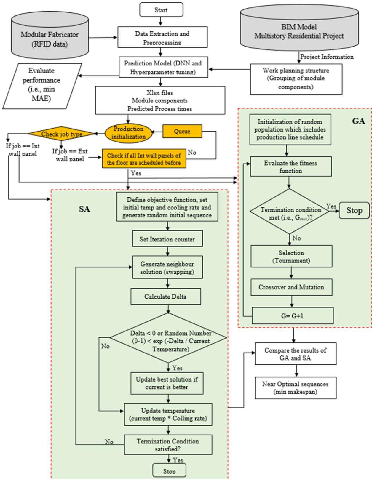
Figure 3.14: Flowchart for scheduling based on GA and SA
