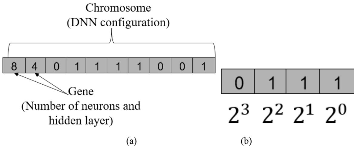
Figure 3.8: (a) Structure of the chromosome; and (b) Decoding of chromosome (learning rate)
