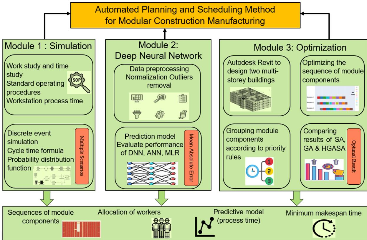
Figure 3.1: Main components of the developed method
