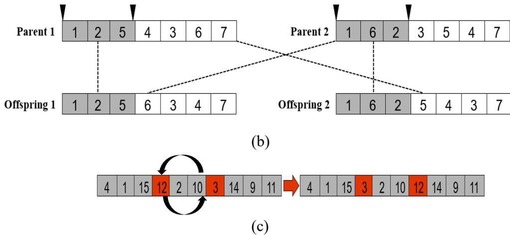
Figure 3.12:(a) Chromosome for module components; (b) two-point Crossover; and (c) swap mutation
