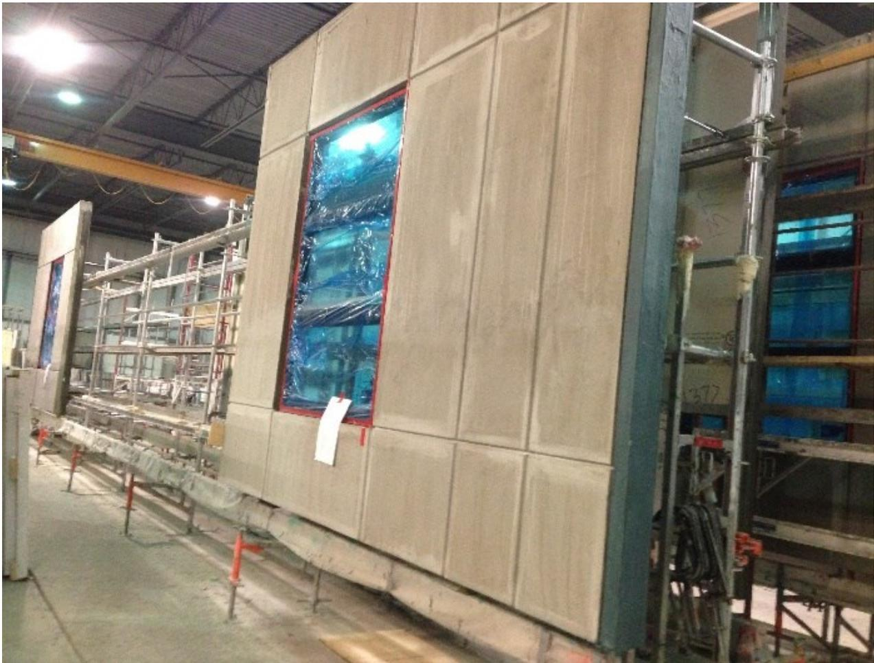
Figure 4.5: Exterior finishing and storage workstation
