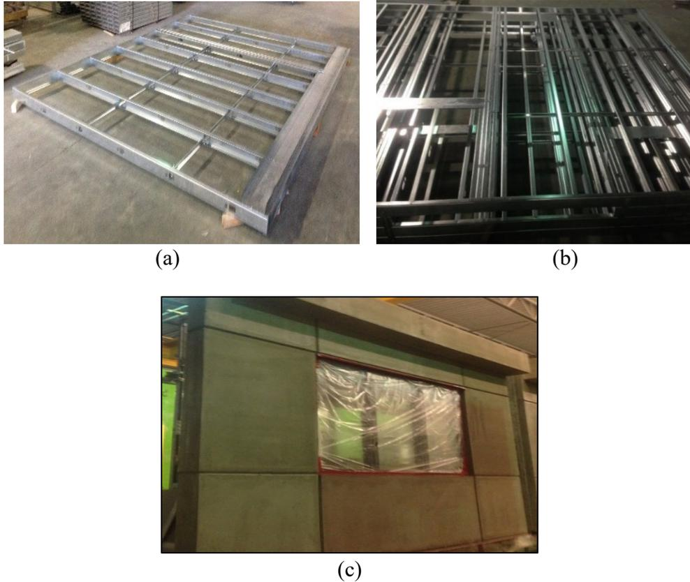
Figure 1.2: Different types of wall panels: (a) Interior wall panel; (b) Interior wall panel with door; and (c) Exterior wall panel with window
