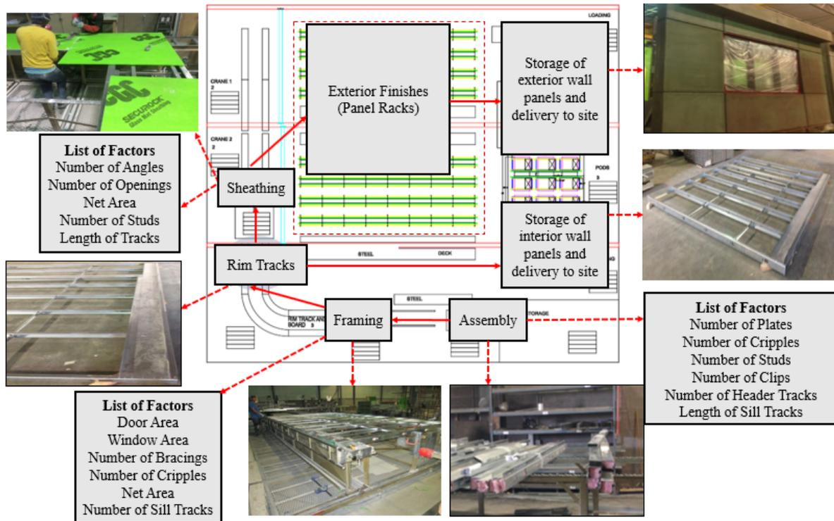
Figure 4.1: Light gauge steel (LGS) wall panel production line
