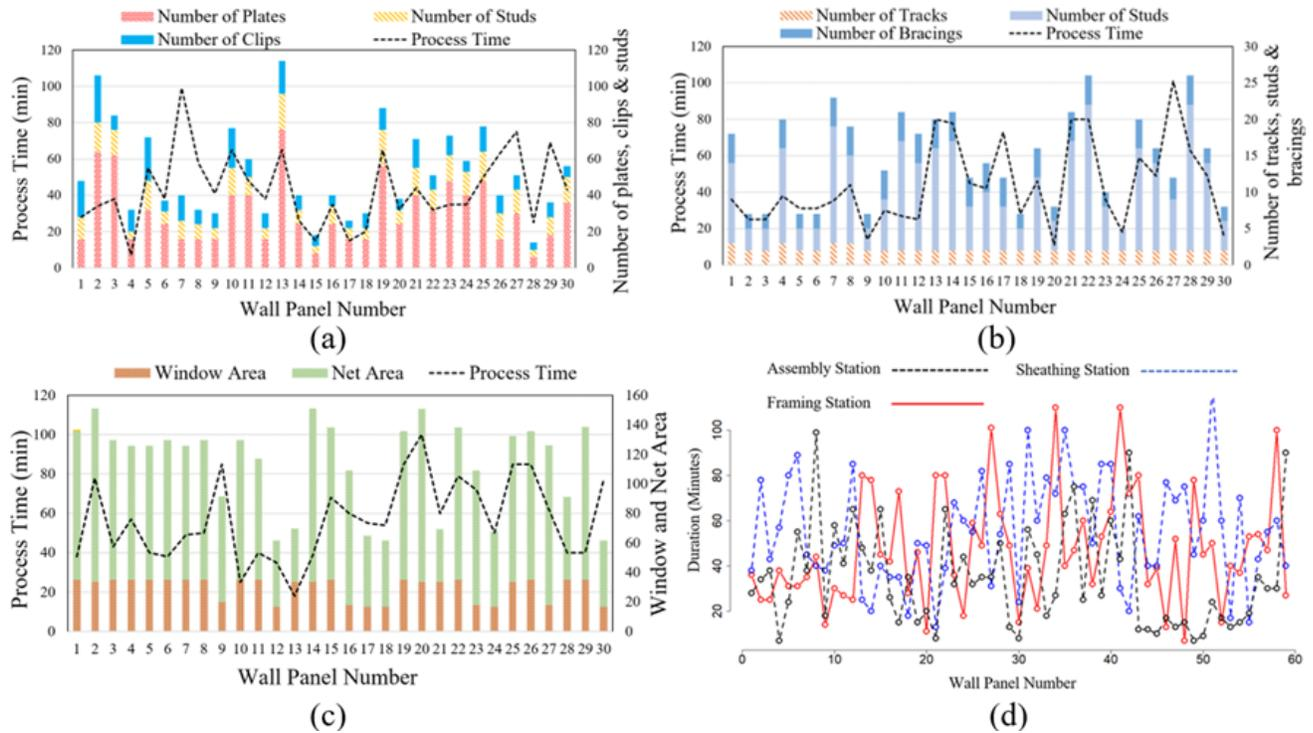
Figure 4.6: (a,b,c): Effect of design specifications on process time, and (d) average productivity of workstation
