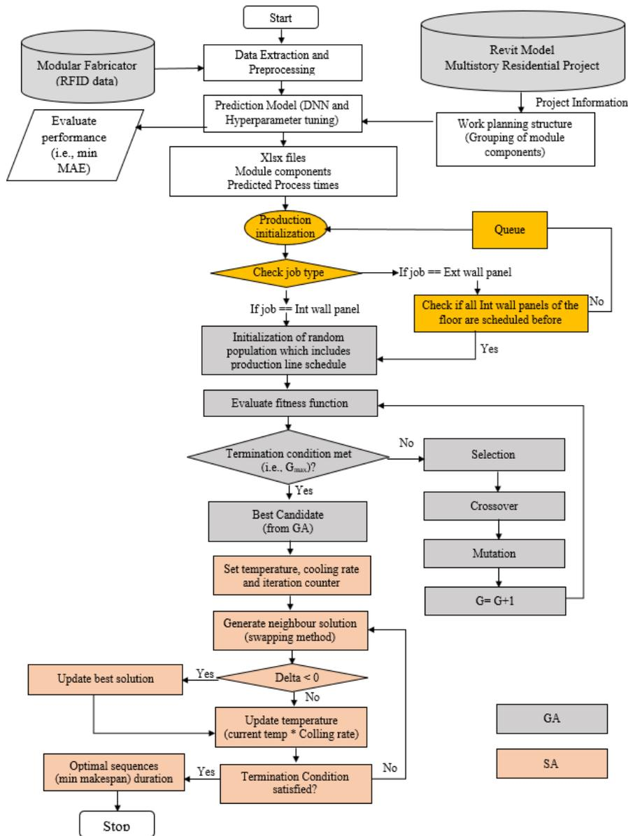
Figure 3.15: Flowchart for scheduling based on Hybrid GASA
