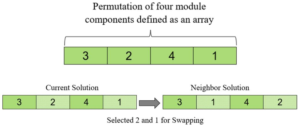
Figure 3.13: Module components defined as an array and neighborhood generation.
