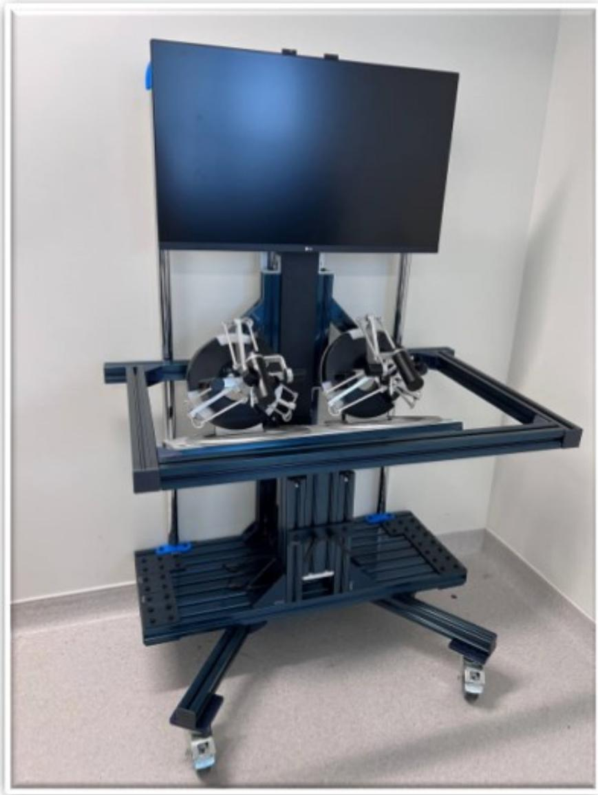
Figure .2: The surgeon console designed, assembled, and used in the robot-assisted laparoscopic system developed in this research.
