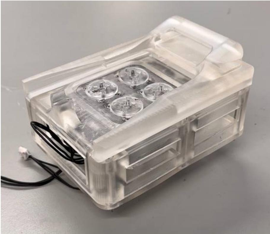
Figure .3: The Adapter designed, 3D printed in-house, and used in the Follower Module: Integration with 4 Dynamixel Motors as the Main Actuation Unit for Surgical Tool Control.
