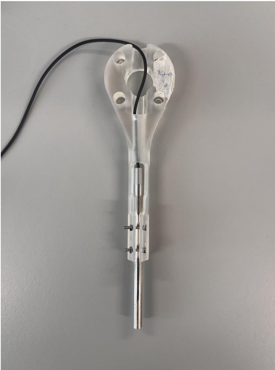
Figure .4: The laparoscope holder designed, fabricated, and used in the Follower Module: a flange to connect the laparoscope to Kinova robotic arms.
