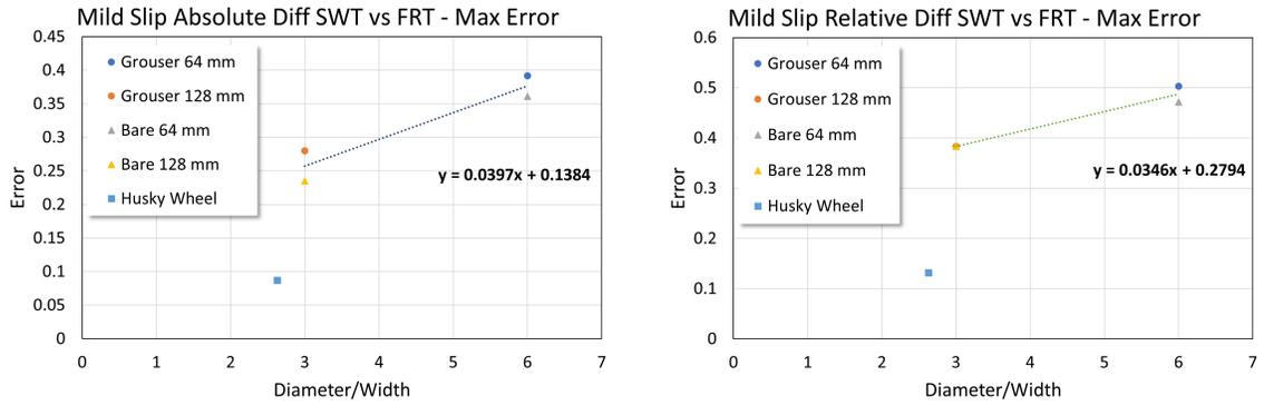
(a) Absolute Error Metric for Grouser Wheel (b) Relative Error Metric for Grouser Wheel
