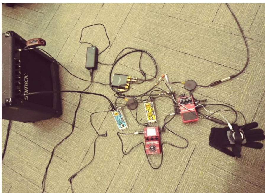
Figure 8 Assemblage of Burur Device: guitar amp, Bluetooth connectors, guitar pedals, transducer and mini amp.
