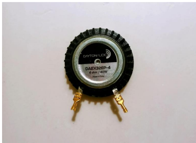
Figure 9 Dayton Audio Exciter (Bass shaker transducer) the component attached to the back of my glove)
