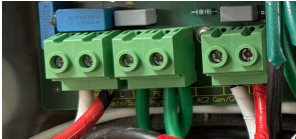
Figure 4-3: power terminals of SI
