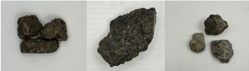
FIGURE 4: RECYCLED CONCRETE AGGREGATE PARTICULES
