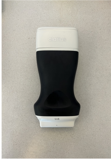
Figure 1.2: Clarius probe. We used this pocket-sized ultrasound device for the collection of patient data in Chapter 4.
