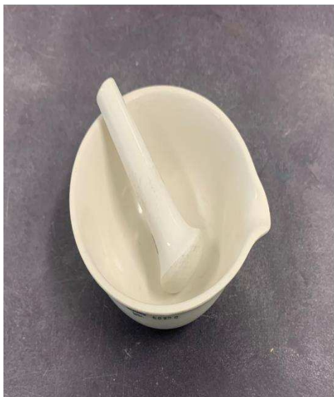
Figure 11. Images of common grinding and milling tools and machines. (A) Mortar and pestle. (B) Planetary ball miller.
