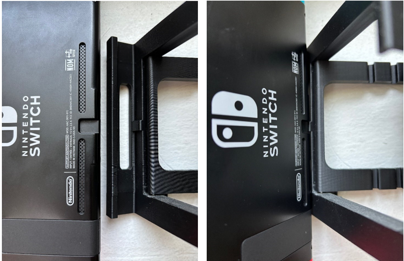
Figure 28 — Showing the small divet in the back of the Switch that allowed for the screen holder the attach.
