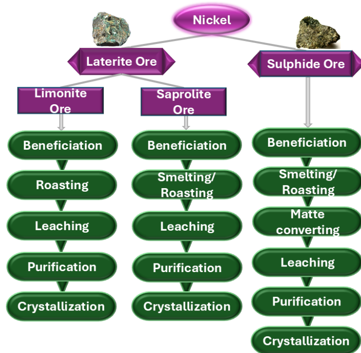
Figure 3: General overview of extraction process of battery-grade materials from nickel from laterite and sulfide ores
