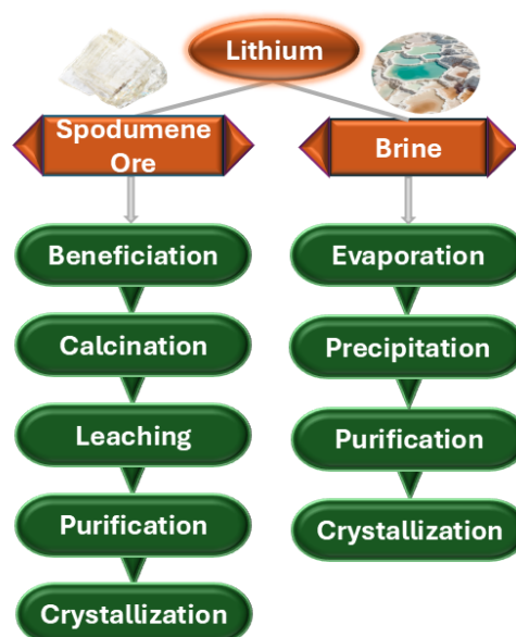
Figure 2: General overview of extraction process of battery-grade materials from lithium from spodumene and brine
