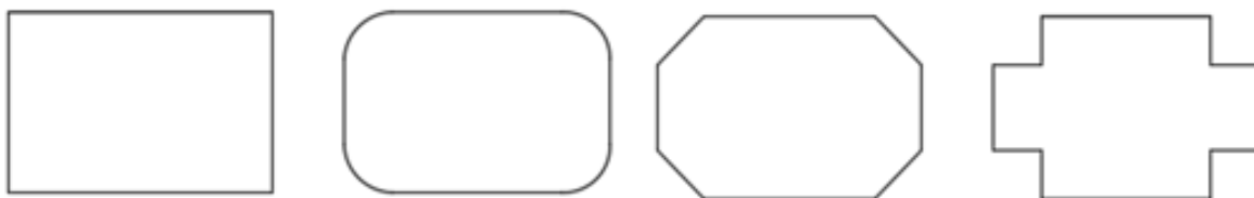
Figure 2.1: Plan shapes of buildings, after Jamieson et al. (1992).
