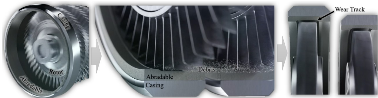
Figure 2.1. Schematic representation of blade–abradable interaction in a gas turbine engine. Adapted from [47].
