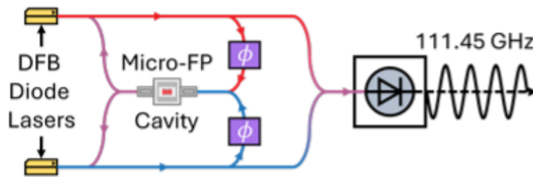
Figure 2.15. Simplified schematic of dual self-injection locking system. [30]
