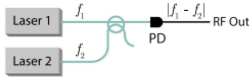
Figure 2.14. Block diagram of mmWoF system with two free-run lasers. [29]
