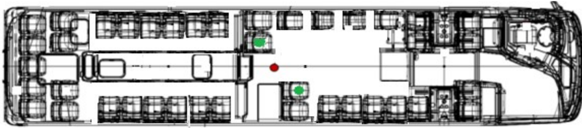
a. Measurement positions considered for noise (in red) and vibration (in green)
