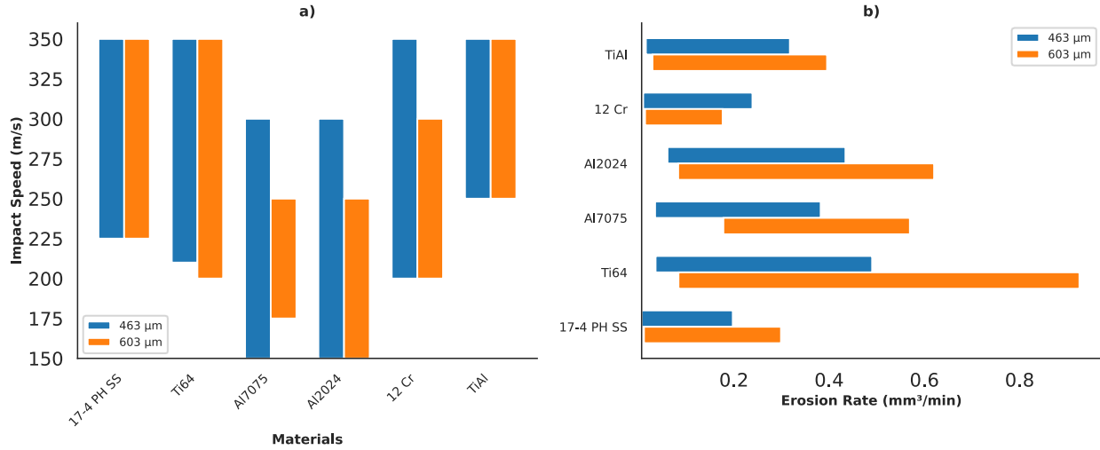
Figure 4.3. a) Impact speed ranges for the tested materials at two different droplet sizes, b) Maximum erosion rates for different materials and droplet sizes
