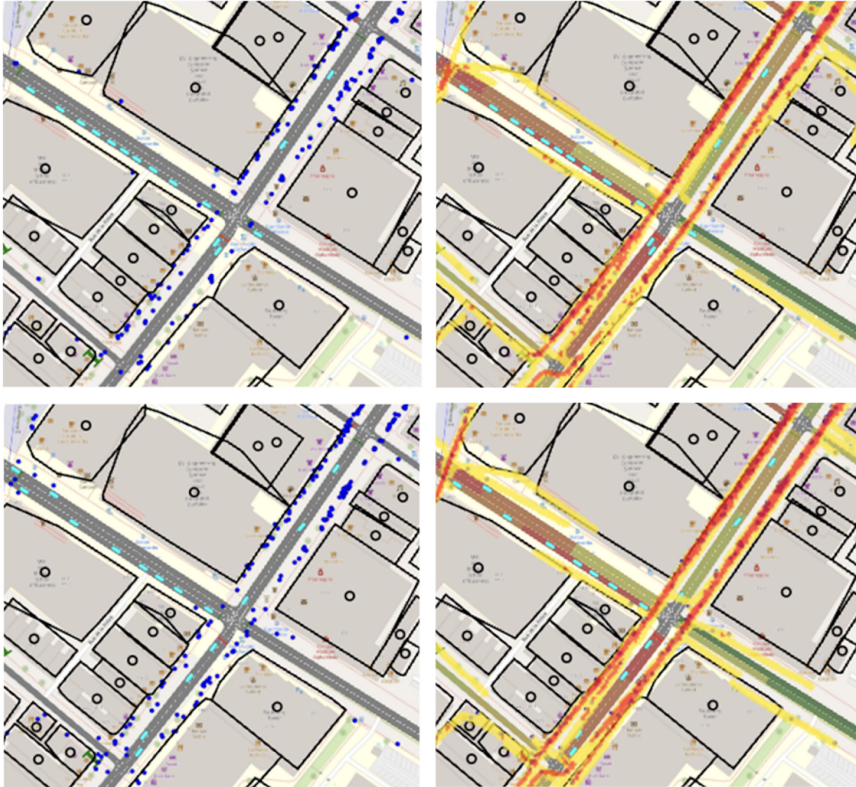
Figure 66 - Agent positions with resulting vehicle speed maps pedestrian heat maps for runs #9 (top) and #10 (bottom)
