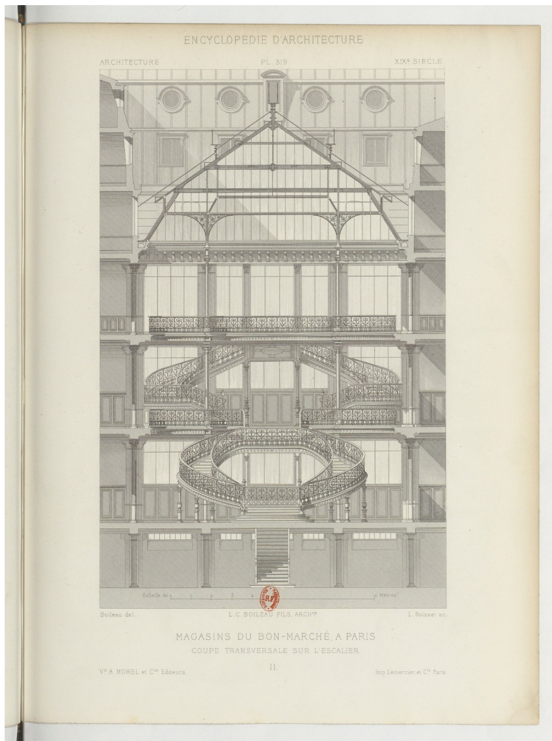
Figure 19. Louis-Charles Boileau (architect), Magasins du Bon Marché, Grand Escalier and the Delicate Wrought-Iron Galleries , 1876. Architectural plans. Encyclopédie d'architecture , vol. 5, 1876, A. Morel, Paris.
